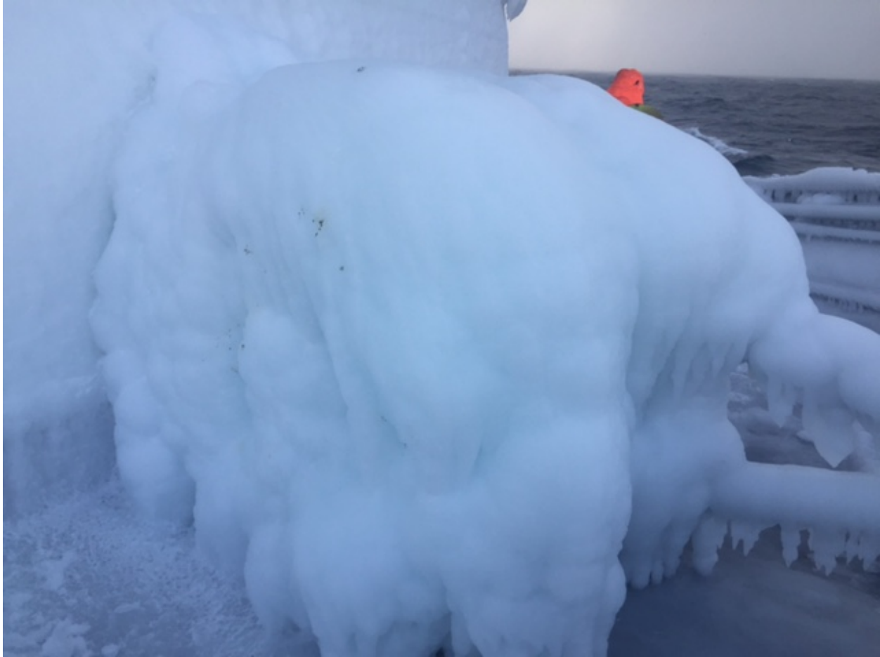
Figure 36 – Photo taken by the Captain of the F/V POLAR SEA of ice accumulation during the transit towards St. Paul Island on February 10
