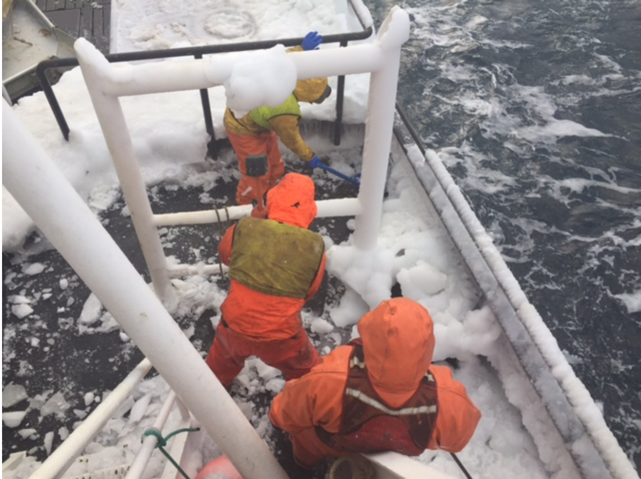
Figure 33 – Photo taken by the Captain of the F/V POLAR SEA of ice accumulation during the transit towards St. Paul Island on February 10
