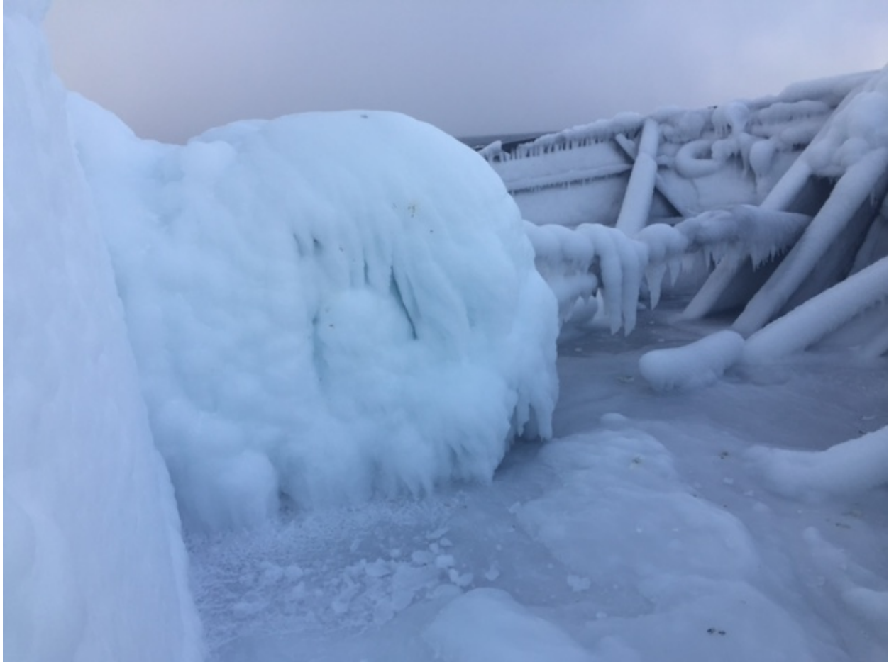
Figure 34 – Photo taken by the Captain of the F/V POLAR SEA of ice accumulation during the transit towards St. Paul Island on February 10
