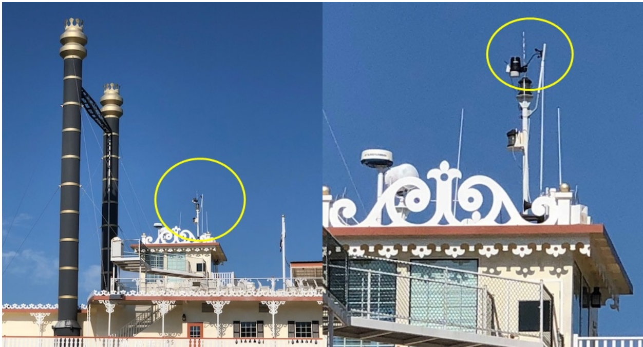
Figure 16 – Photos of the Showboat Branson Belle's anemometer taken two days after the Stretch Duck 7 accident.
