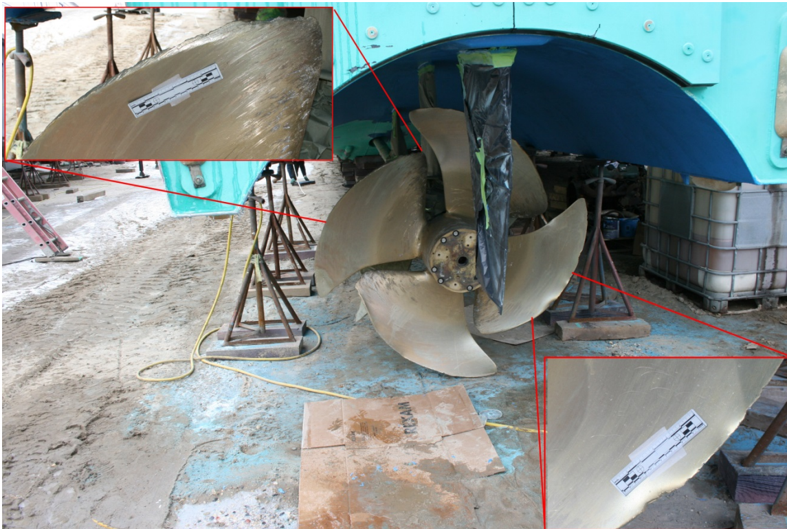
Figure 12. Port propeller blade damage. Photo insets show the close up view of the damage to two of the propeller blades.
