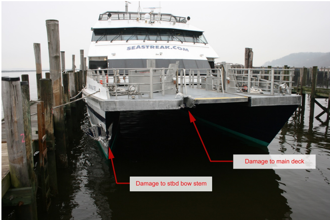
Figure 11. Damage to starboard bow stem and main deck.
