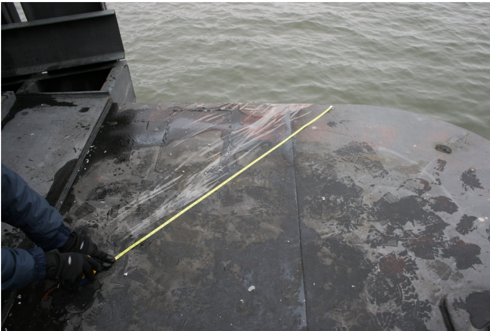
Figure 14. Scratches on deck of deck barge, at an approximate angle of 45° to top edge of the headlog.
