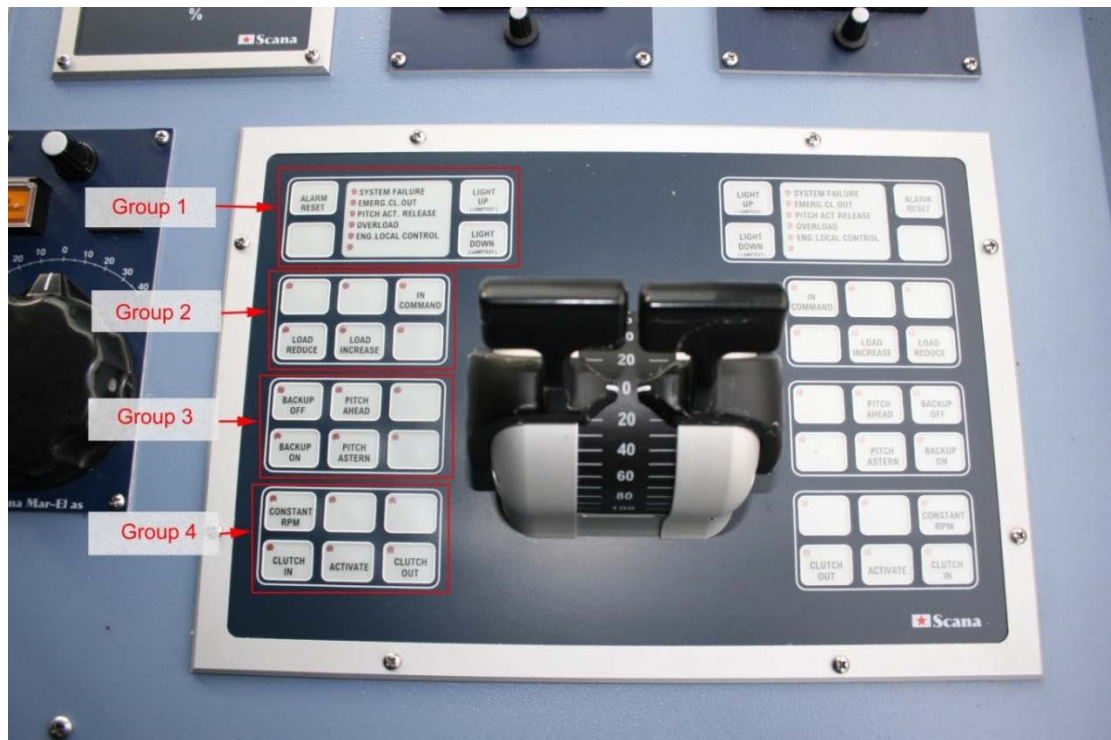
Figure 6. Propulsion control panel button grouping.
