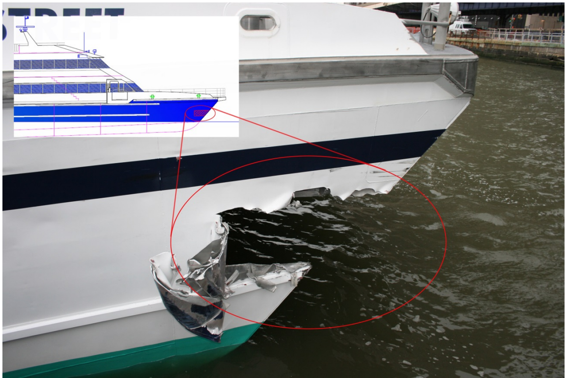
Figure 9. Damage to stem of starboard hull
