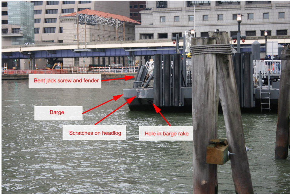
Figure 13. Damage to deck barge and sideloader.
