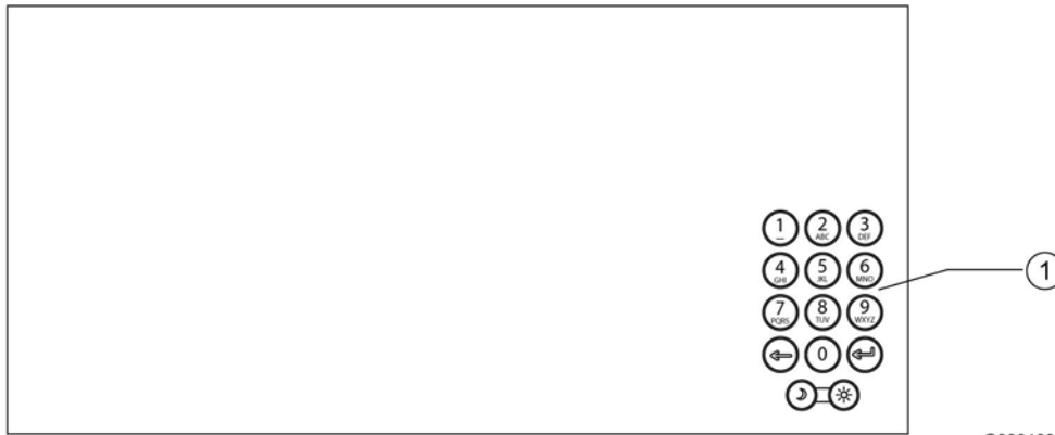
Figure 6. The keypad on the control panel.
