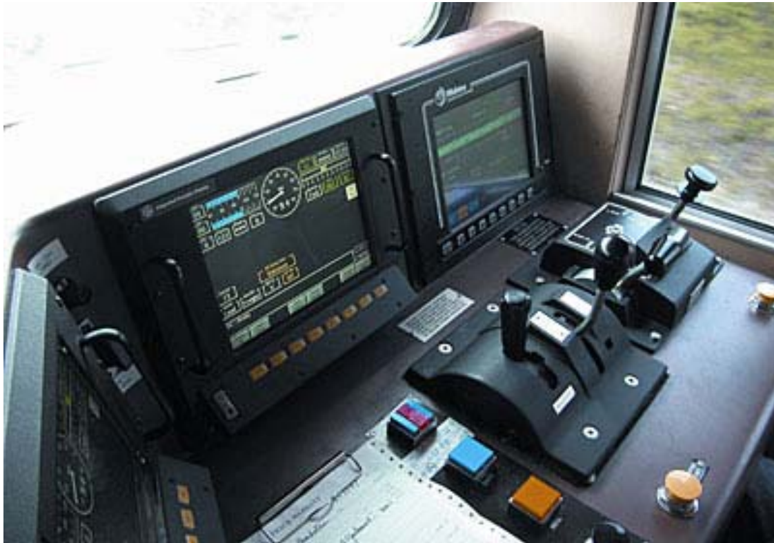
Figure 6: Locomotive Control Display (Left) and I-ETMS Display (Right)
