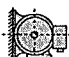
IM B6 IM 1051 foot wall mounted with feet on left-hand side when viewed from DE
