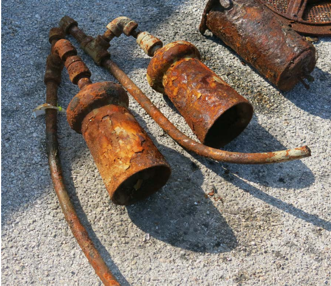
Figure 7. Discharge nozzles for fixed fire suppression system.
