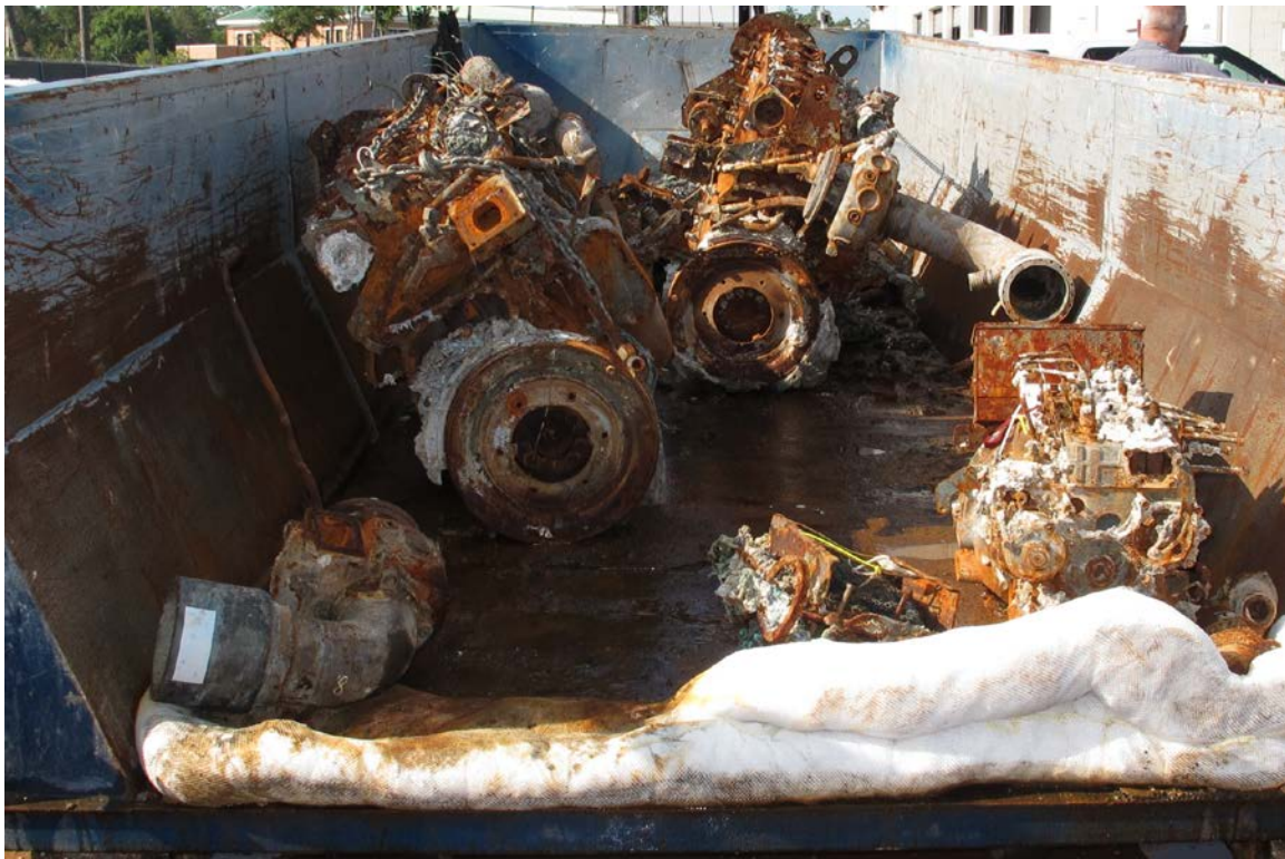
Figure 2. Portions of the starboard (right) and port (left) engines after recovery.
