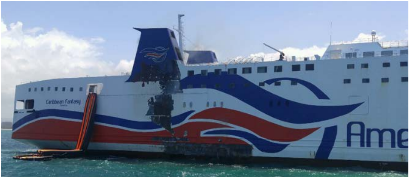
Figure 26. Photograph of starboard side of ship on August 19. Smoke can be seen coming from the exhaust stacks on the upper deck.
