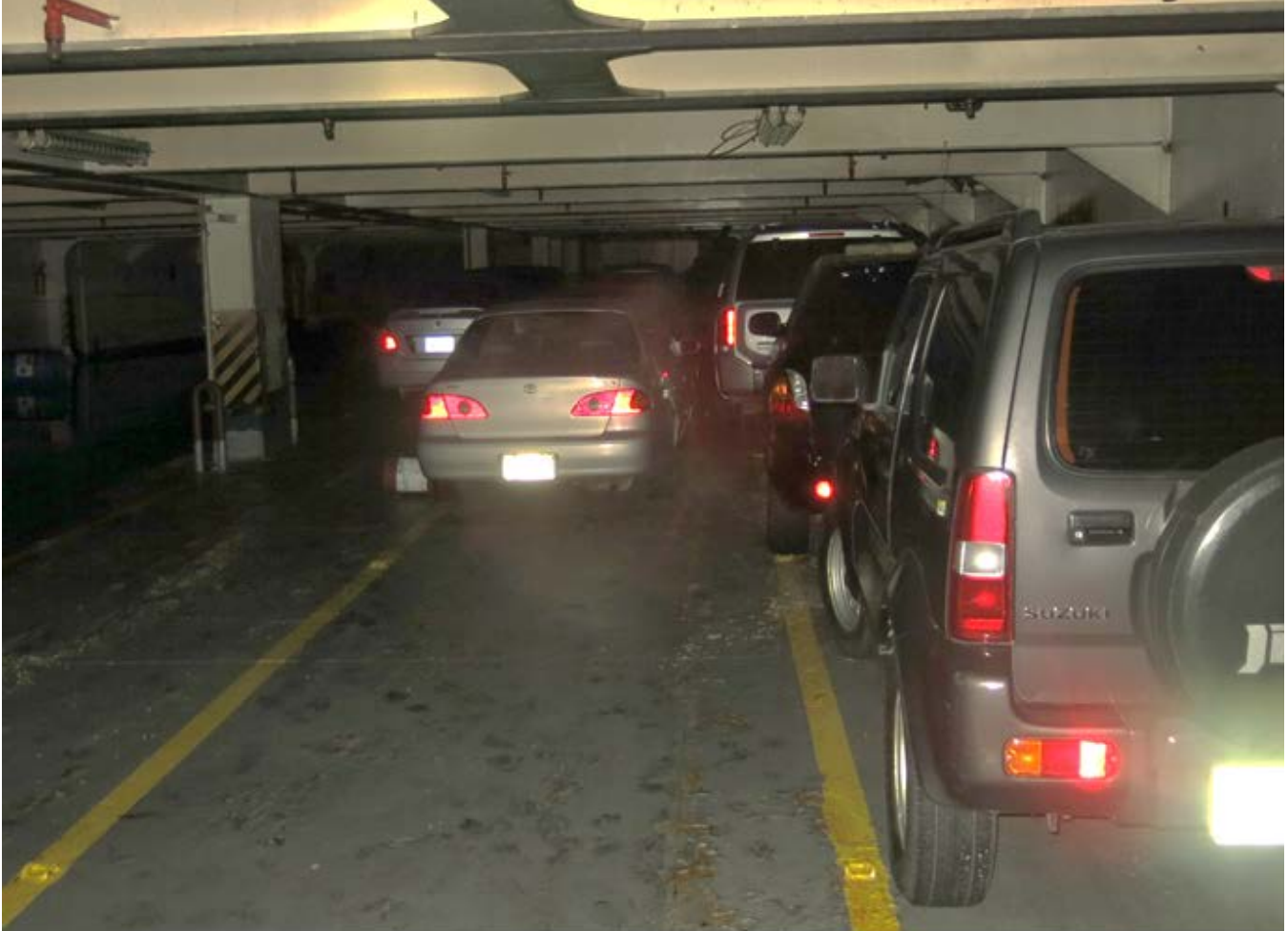
Figure 33. Overall photograph of Garage Deck A (Deck 2) facing forward. Water can be seen on deck on the left side of the image.
