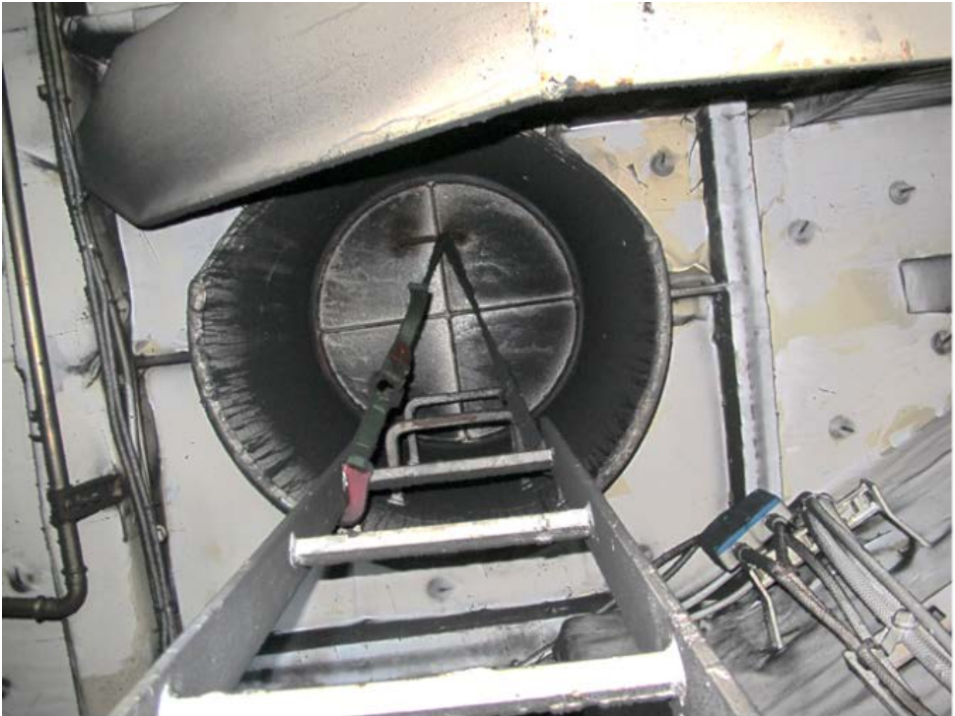
Figure 8. Photograph of upper hatch of CO 2 room to the deck 4 aft mooring deck with strap securing hatch from inside the space.
