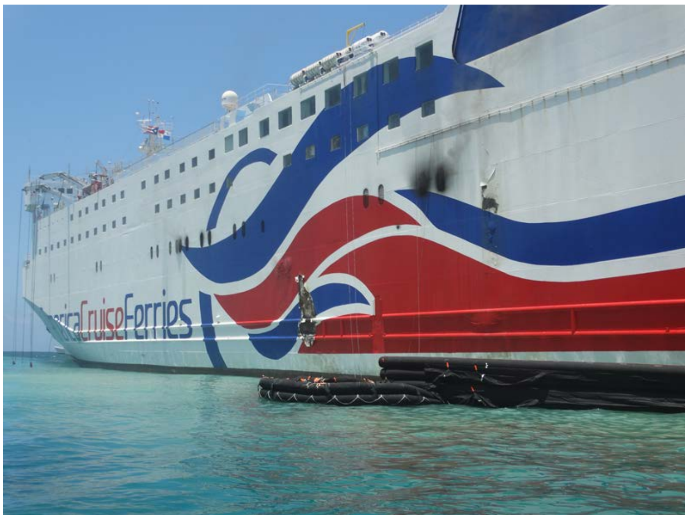
Figure 23. Photograph of port side of ship at 1308 on 8/17/16. No hull damage shown. Paint starting to discolor forward of bunker stations door.
