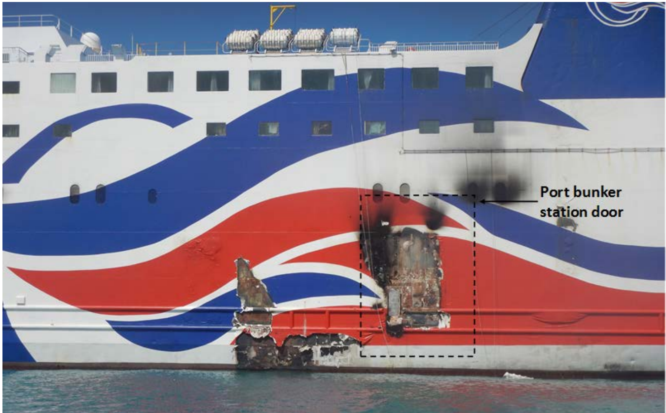
Figure 4. Photograph of port side of ship at 1512 on 8/18/16. Paint on bunker station door has burned away.
