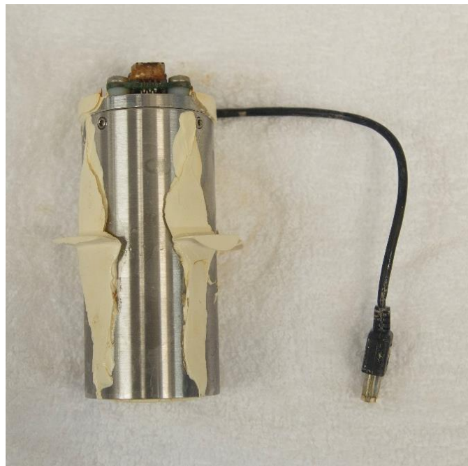
Figure 8. Inner capsule assembly after removal from VDR capsule.
