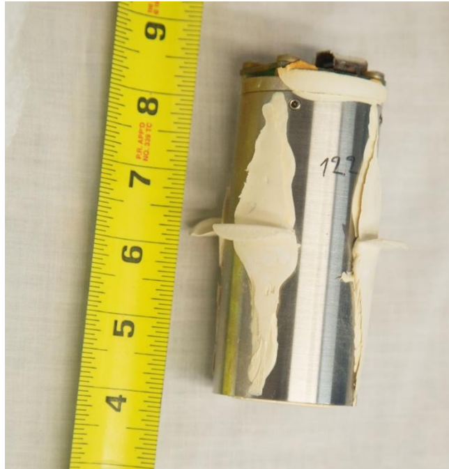
Figure 9. Inner capsule assembly after removal from VDR capsule.
