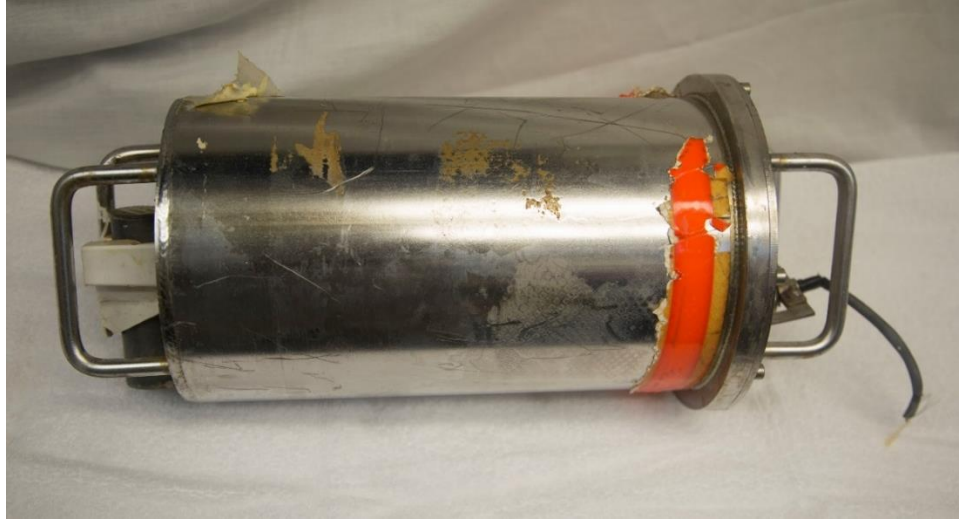
Figure 7. VDR capsule before disassembly.
