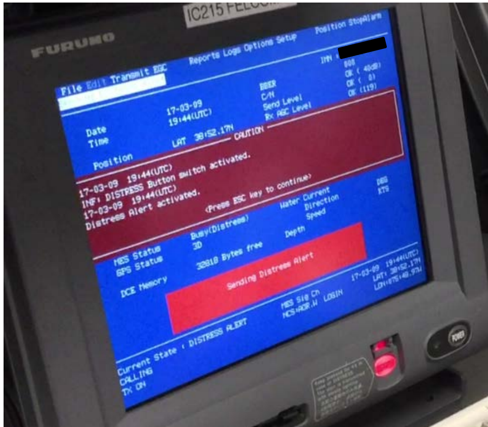
Figure 5. Furuno FELCOM 15 distress alert activation.
