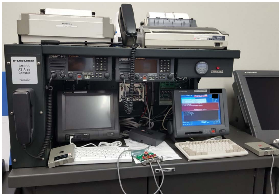
Figure 1. The Furuno FELCOM 15 terminal (lower right) and printer (upper right) used during test.
