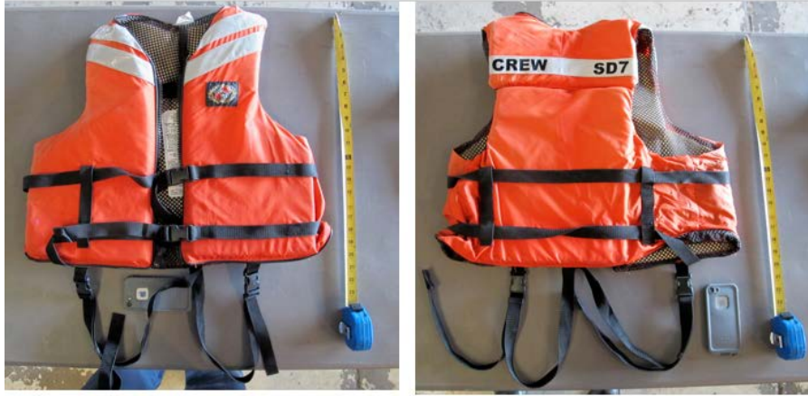
Front and back of the Type III adult flotation vest carried on board the Stretch Duck 7
