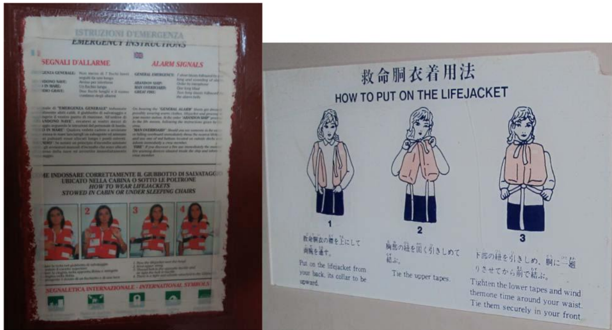
15 16 Figure 1. Left: Emergency instruction sign, in English and Italian, on the back of a deck 6 cabin 17 door. The fire instructions are also incorrect as they state in case of a “great fire” the signal is “two 18 long blasts followed by the alarm bells.” Also note the masking tape covering the outer edges of 19 the emergency instructions. Right: Lifejacket donning instruction sign, in English and Japanese, 20 found on deck 6 near fire locker no. 2. The instructions are not for the lifejacket types carried on 21 board at the time of the accident.
