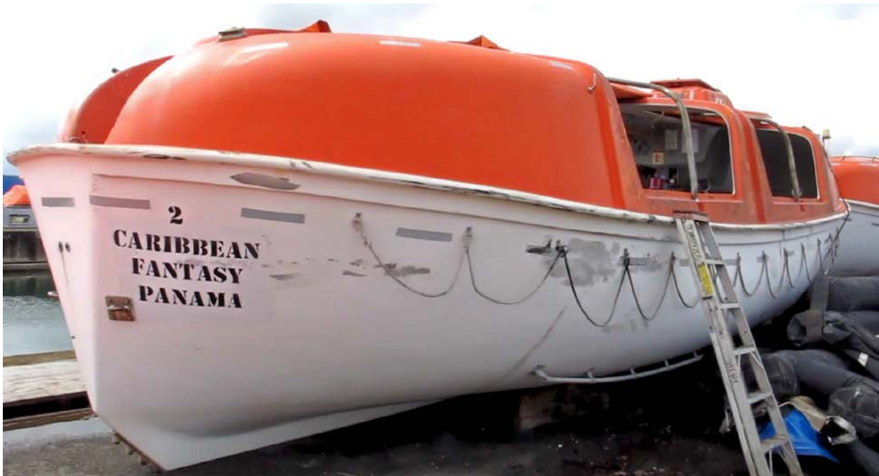
10 11 Figure 1. Caribbean Fantasy lifeboat no. 2 on the pier in San Juan after the accident. Canvas tarps 12 hinged on the top of the lifeboat were designed to cover the entrances on each side of the boat.
