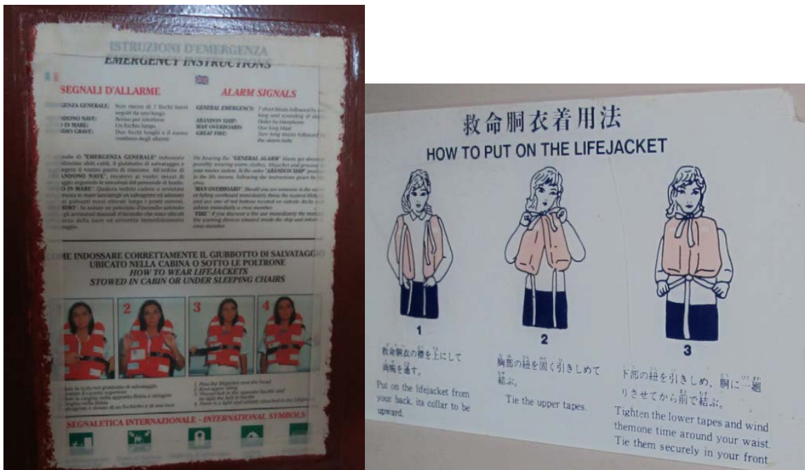
1 2 Figure 24. Left image from the back of a passenger cabin door. Instructions were in Italian and 3 English and stated that the signal for a “great fire” was “two long blasts followed by alarm bells,” 4 which was not a signal used on board. Right image from a public space on deck 7 describing 5 lifejacket donning instructions in English and Japanese for a type of lifejacket not found on board.
