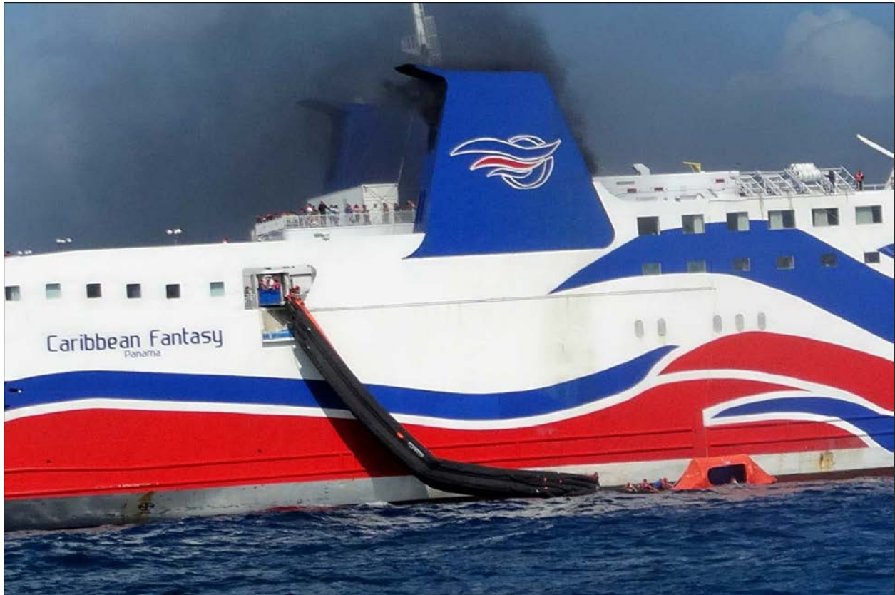
1 2 Figure 13. Caribbean Fantasy starboard side MES deployed with steep angle. Note the large opening 3 of the liferaft is turned away from the MES platform. (Photo by US Coast Guard)
