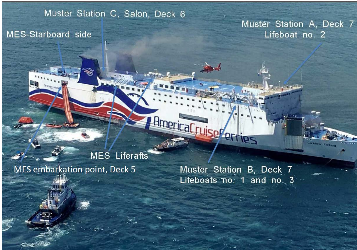
5 6 Figure 16. Muster station, MES, and lifeboat locations on board the Caribbean Fantasy . (Photo by 7 Coast Guard)
