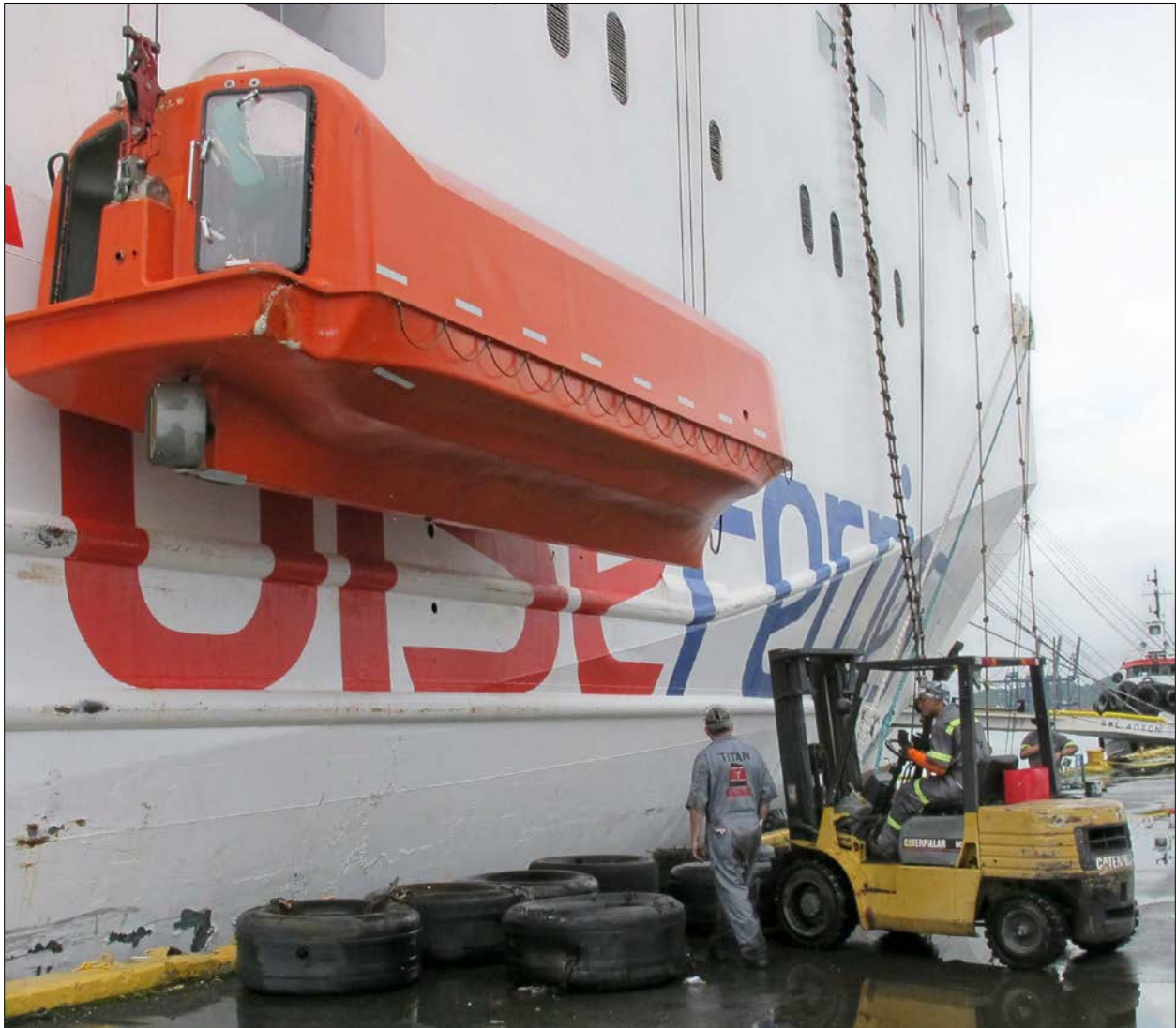
Figure 2. Caribbean Fantasy lifeboat no. 3. Workers prepare the lifeboat so that investigators can exercise the hook release mechanism.
