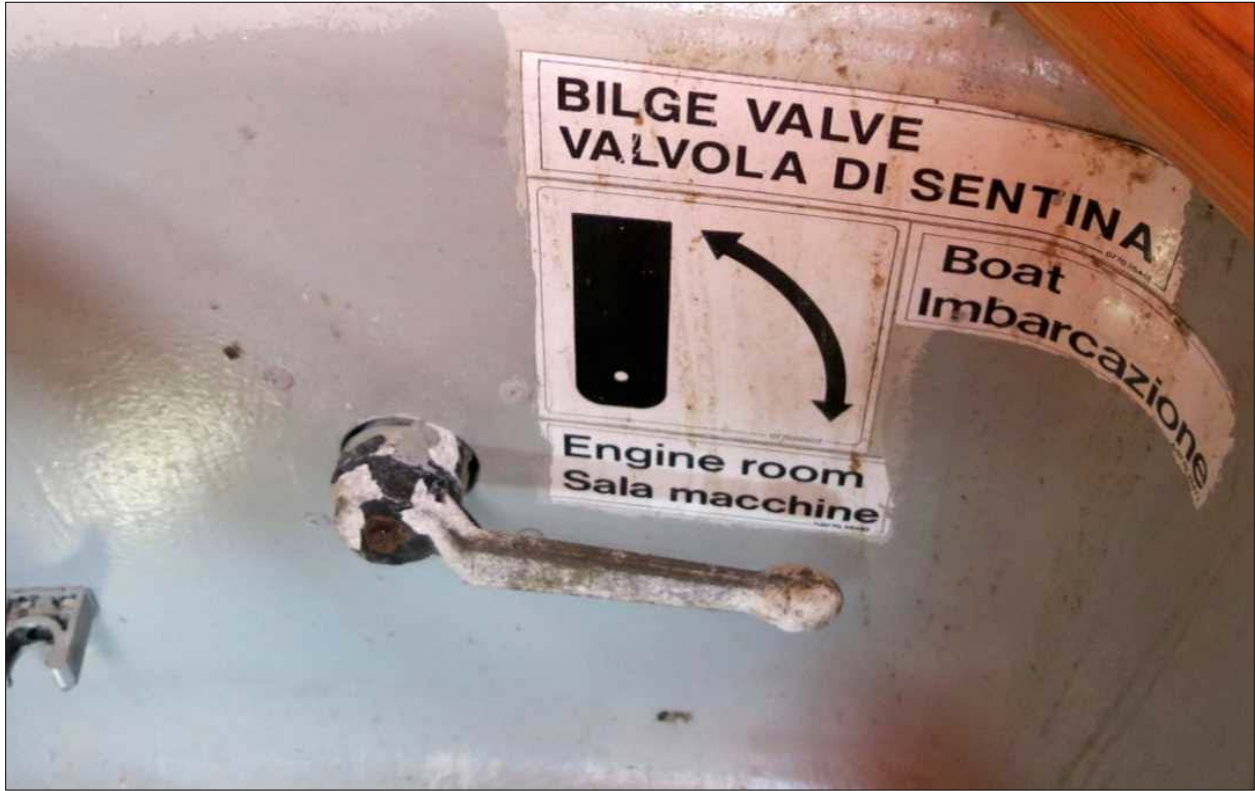
4 5 Figure 27. Caribbean Fantasy lifeboat no. 1 bilge pump valve handle in position to remove water 6 from the engine compartment. Note labels are in English and Italian.
