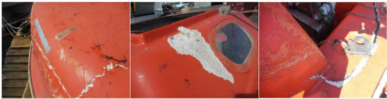
19 20 Figure 28. Damage to lifeboats (Photos courtesy of Palfinger Marine)
