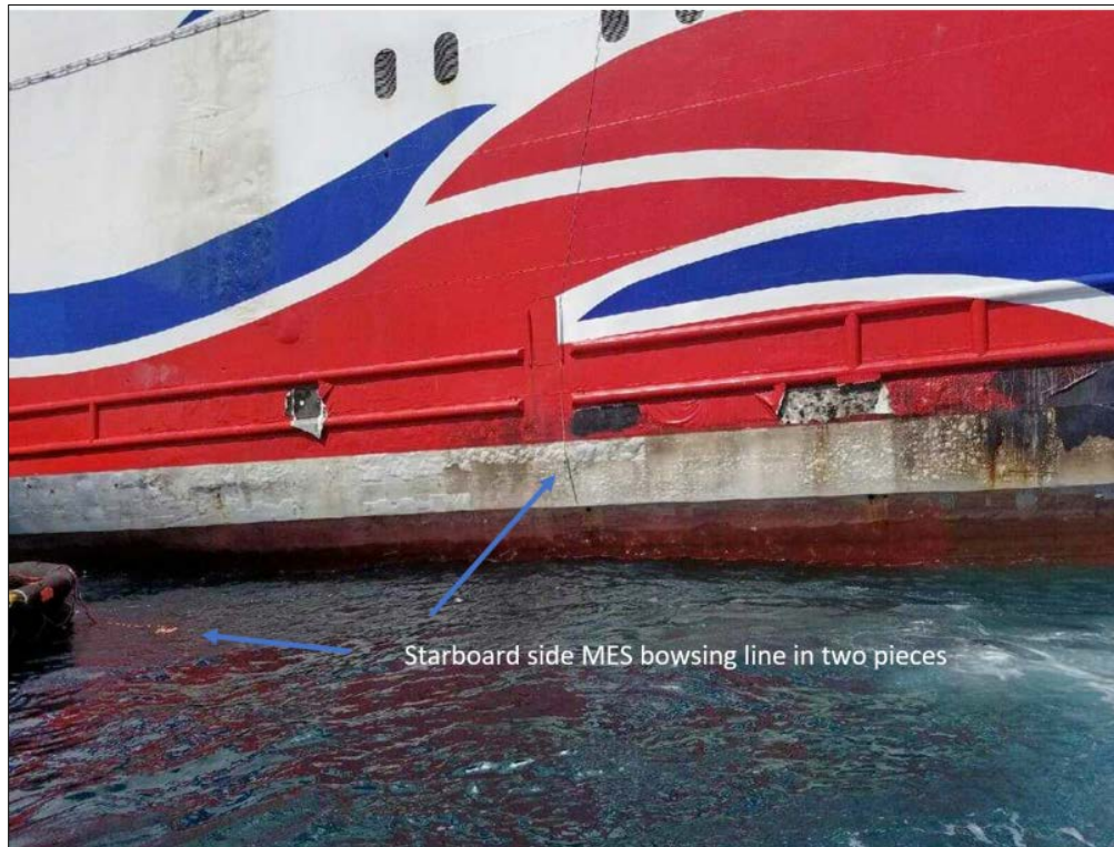
7 8 Figure 12. From left to right: A piece of the bowsing line attached to the starboard side MES 9 platform; and the rest of the bowsing line, hanging slack on the side of the Caribbean Fantasy 10 (Photo by Coast Guard)
