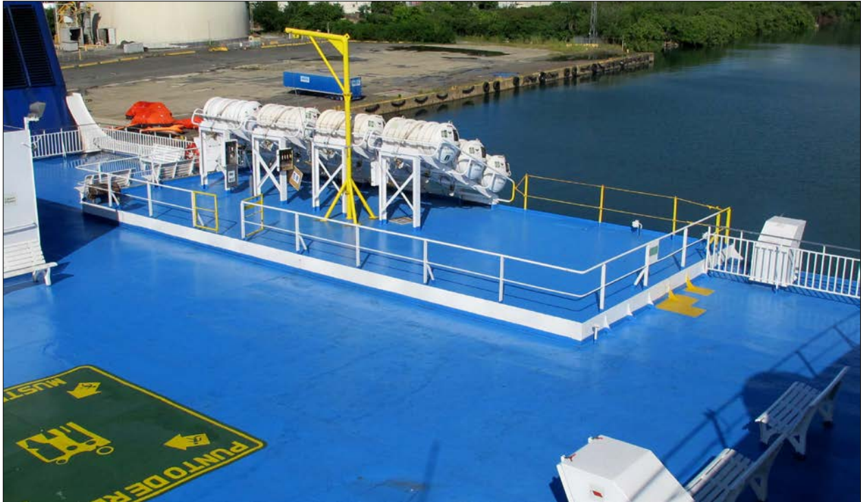
1 2 Figure 7. Postaccident photo of the life raft containers and storage racks for the 3 Caribbean Fantasy's port side marine evacuation system.
