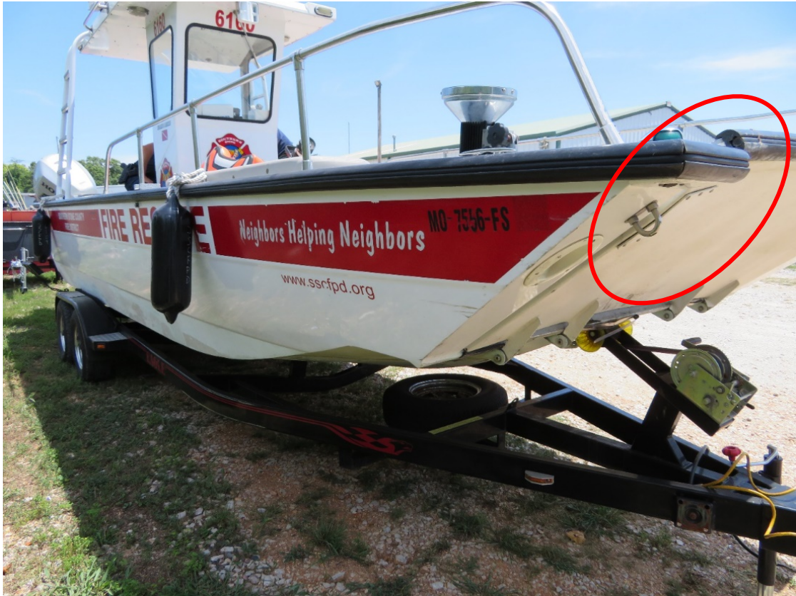
1 2 SSCFPD's boat after the incident with damaged bow ramp, indicated by red circle, and with stress 3 fractures throughout the hull.
