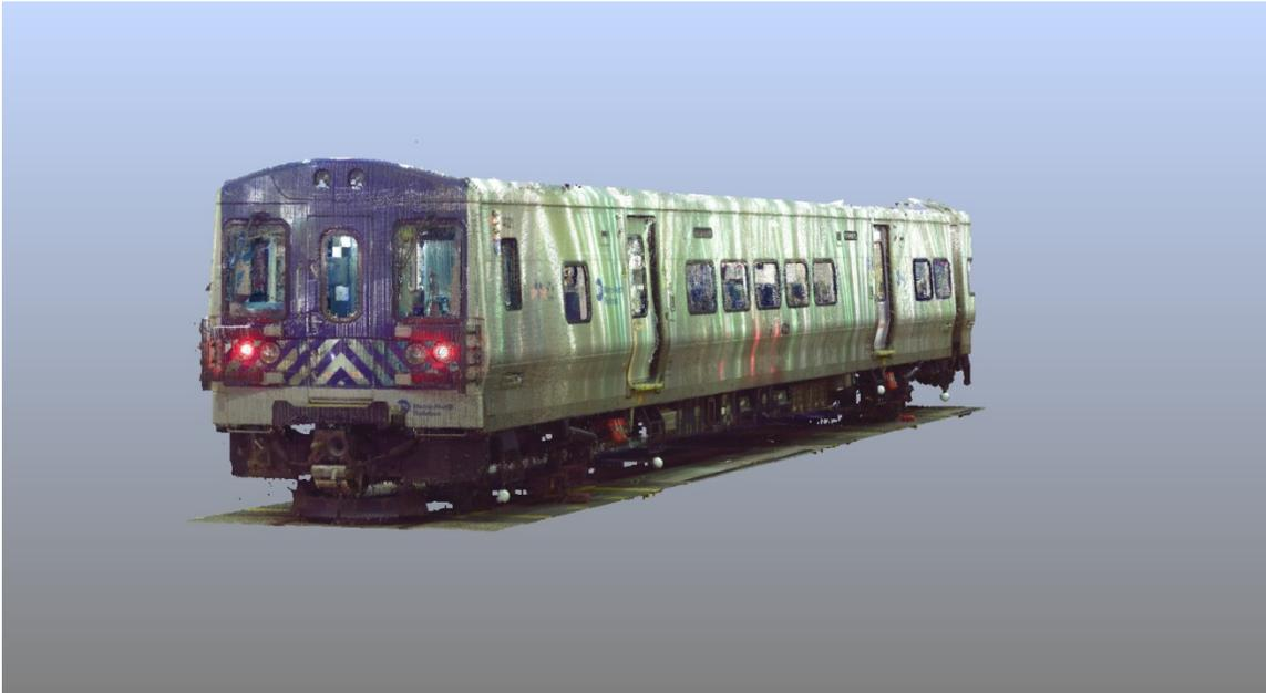
Figure 17: An image from the 3D laser scanner point cloud showing left side of rail car 4021.
