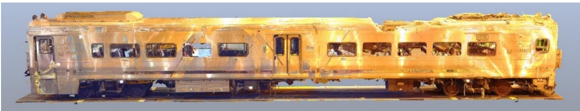
Figure 10: An image from the 3D laser scanner point cloud showing the right side of lead cab car 6036. (The F-end is on the right side of the image.)
