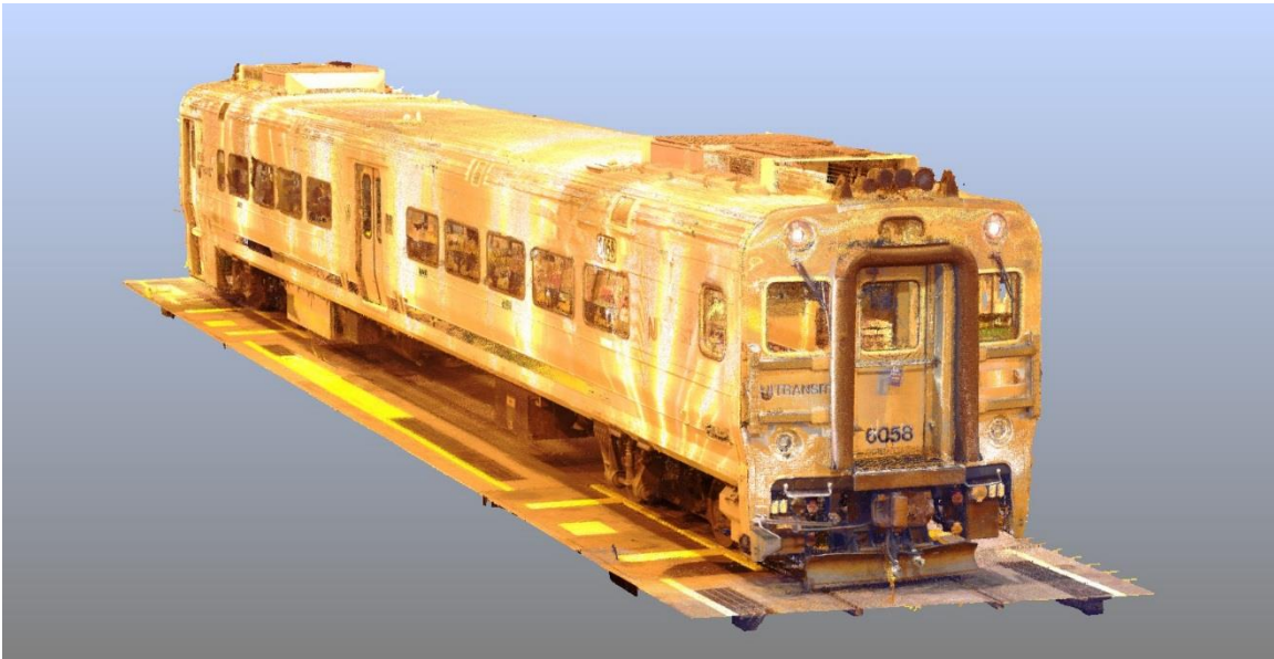
Figure 5: An image from the 3D laser scanner point cloud showing F-end and right side of exemplar cab car 6058.
