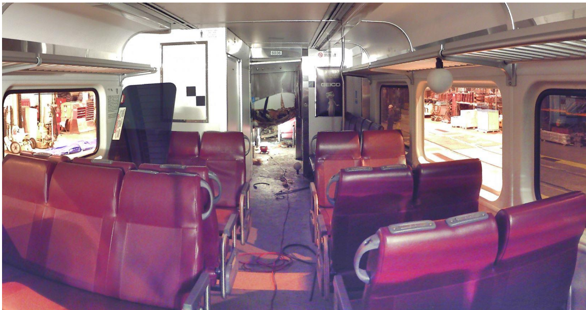
Figure 12: A planar image from the 3D laser scanner showing the rear passenger compartment and the intrusion forward of the center vestibule. The view is looking forward in the direction of train travel.
