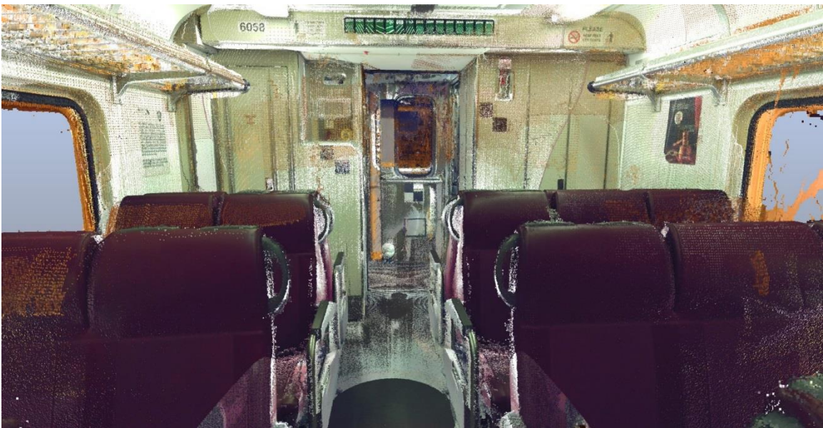
Figure 7: An image from the 3D laser scanner point cloud showing the interior of exemplar cab car 6058.
