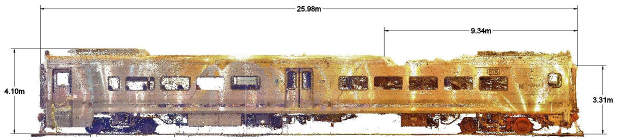
Figure 14: An image from the 3D laser scanner point cloud showing the overall dimensions (in meters) of lead cab car 6036 and the general region of exterior damage. (The F-end is on the right side of the image.)
