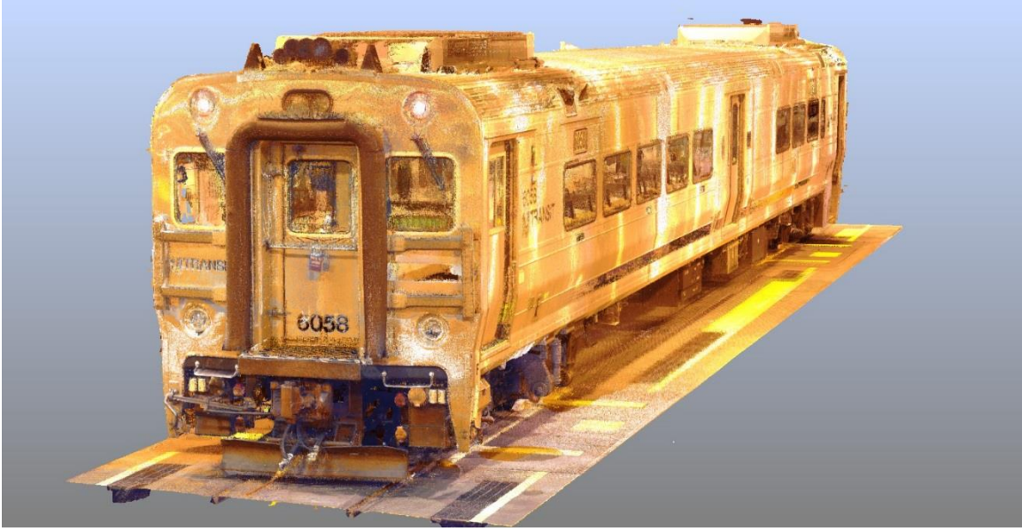
Figure 6: An image from the 3D laser scanner point cloud showing F-end and left side of exemplar cab car 6058.
