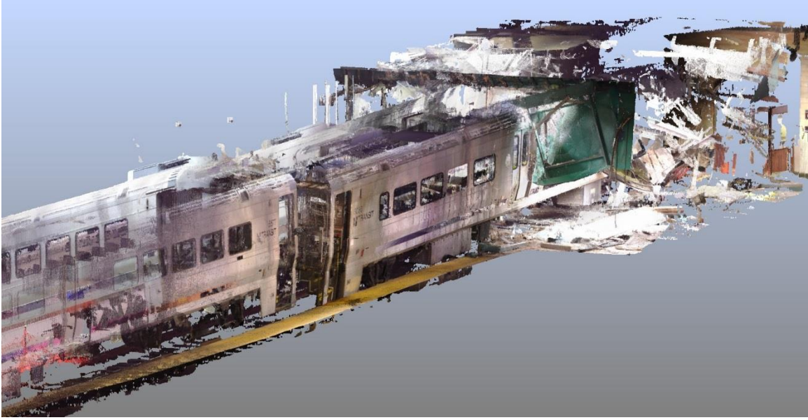
Figure 2: An image from the 3D laser scanner point cloud showing the right side of the cab car and a portion of car 2. The direction of train travel was from the left side of the image toward the right side of the image.
