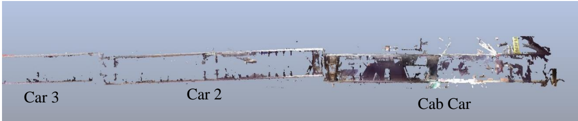
Figure 4: An image from the 3D laser scanner point cloud showing an overhead view of the orientation of the cab car relative to car 2 and car 3. The direction of train travel was from the left side of the image toward the right side of the image.
