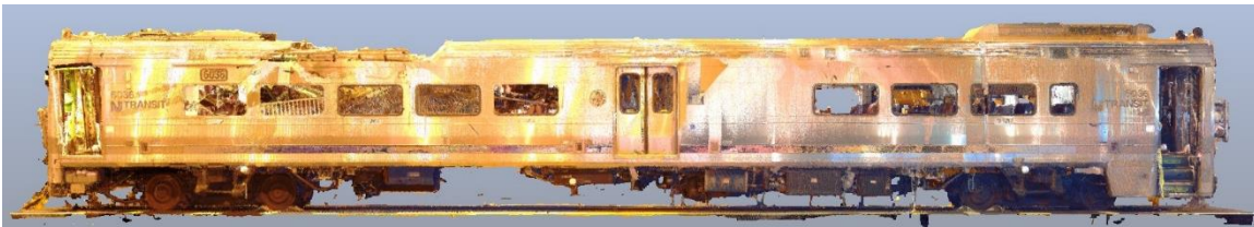
Figure 9: An image from the 3D laser scanner point cloud showing the left side of lead cab car 6036. (The F-end is on the left side of the image.)
