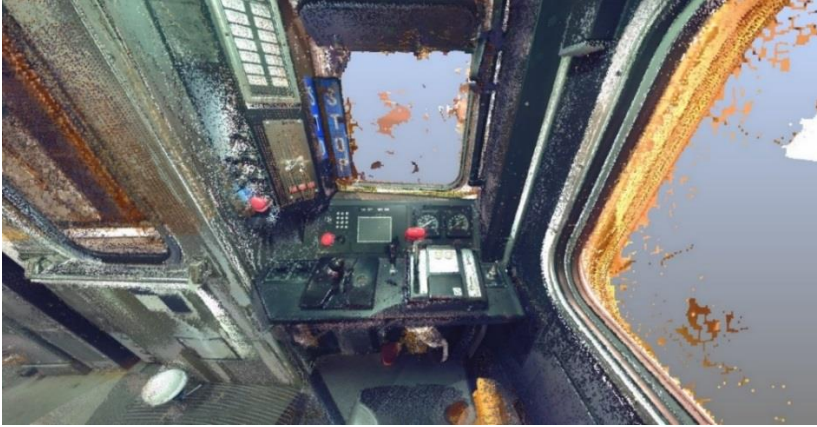
Figure 8: An image from the 3D laser scanner point cloud showing the cab and control console of exemplar cab car 6058.
