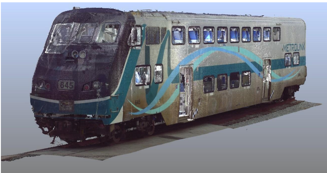
Figure 1: An image from the 3D laser scanner point cloud showing left side of the cab car - 645.
