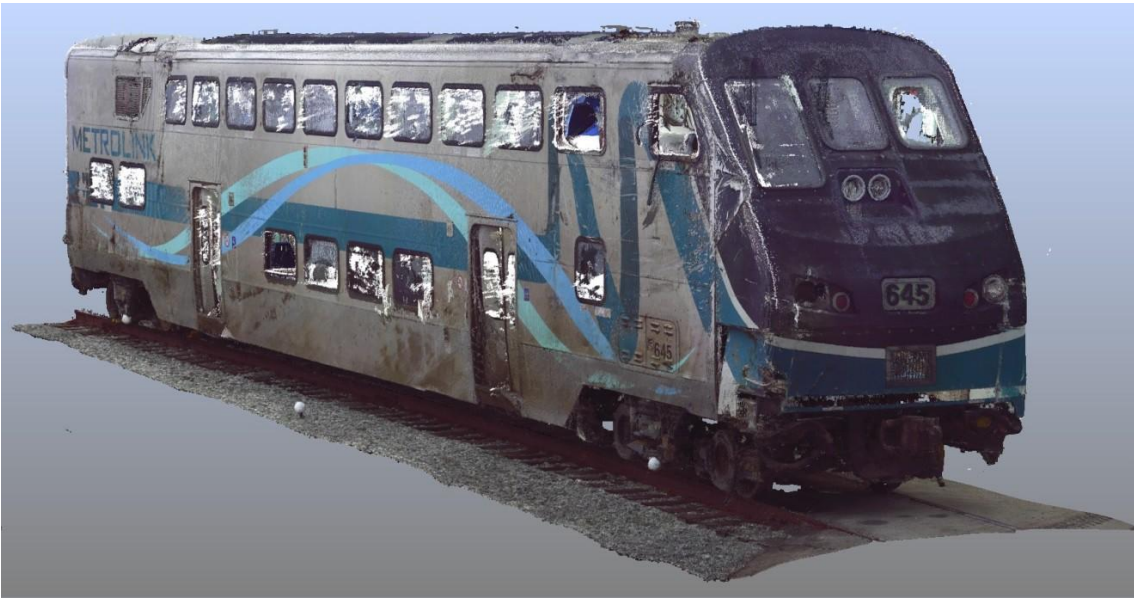
Figure 2: An image from the 3D laser scanner point cloud showing the right side of the cab car - 645.
