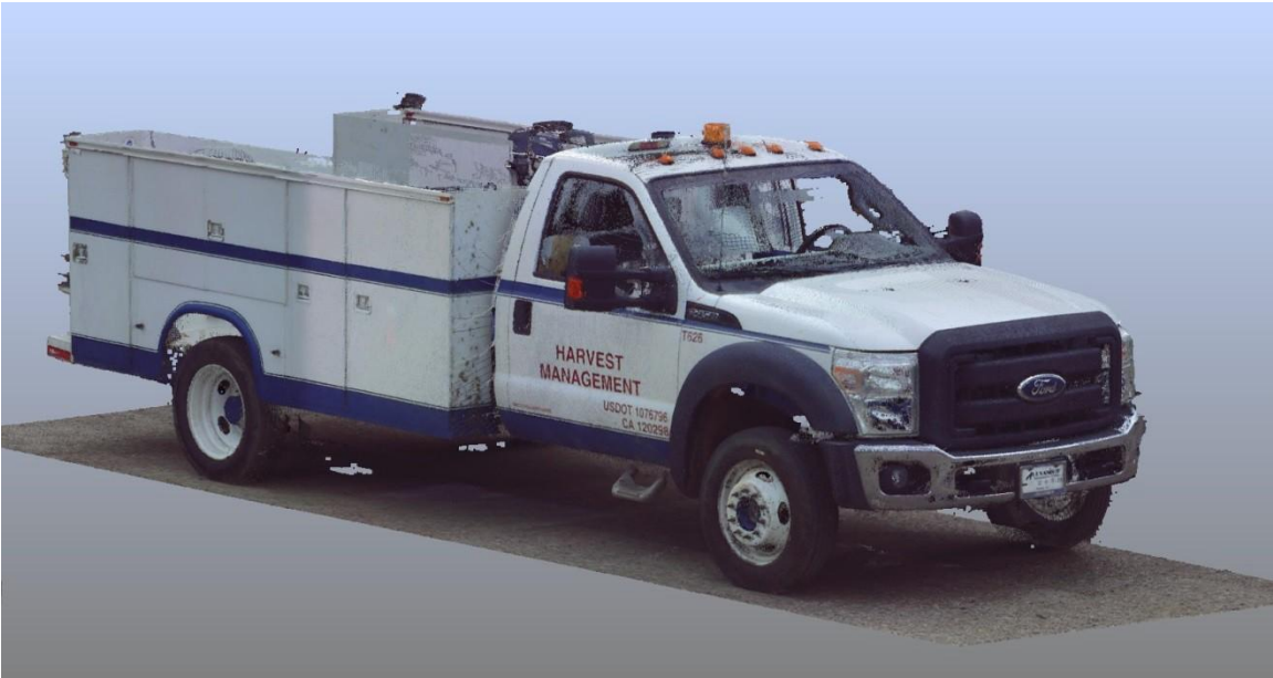
Figure 18: An image from the 3D laser scanner point cloud showing the right side of the 2011 Ford F450.
