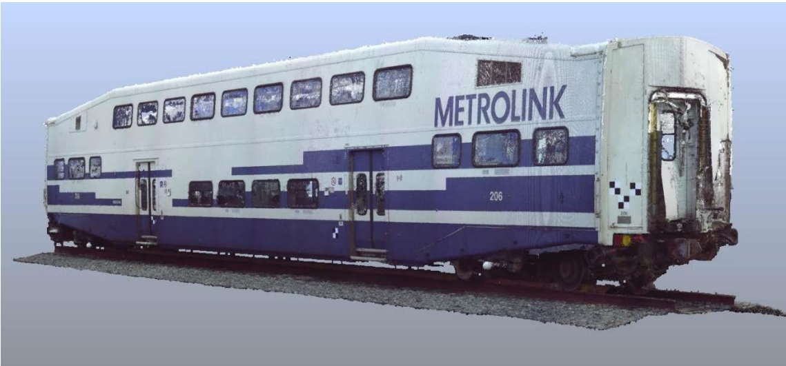
Figure 6: An image from the 3D laser scanner point cloud showing the right side and A end of the 2 nd rail car - 206.
