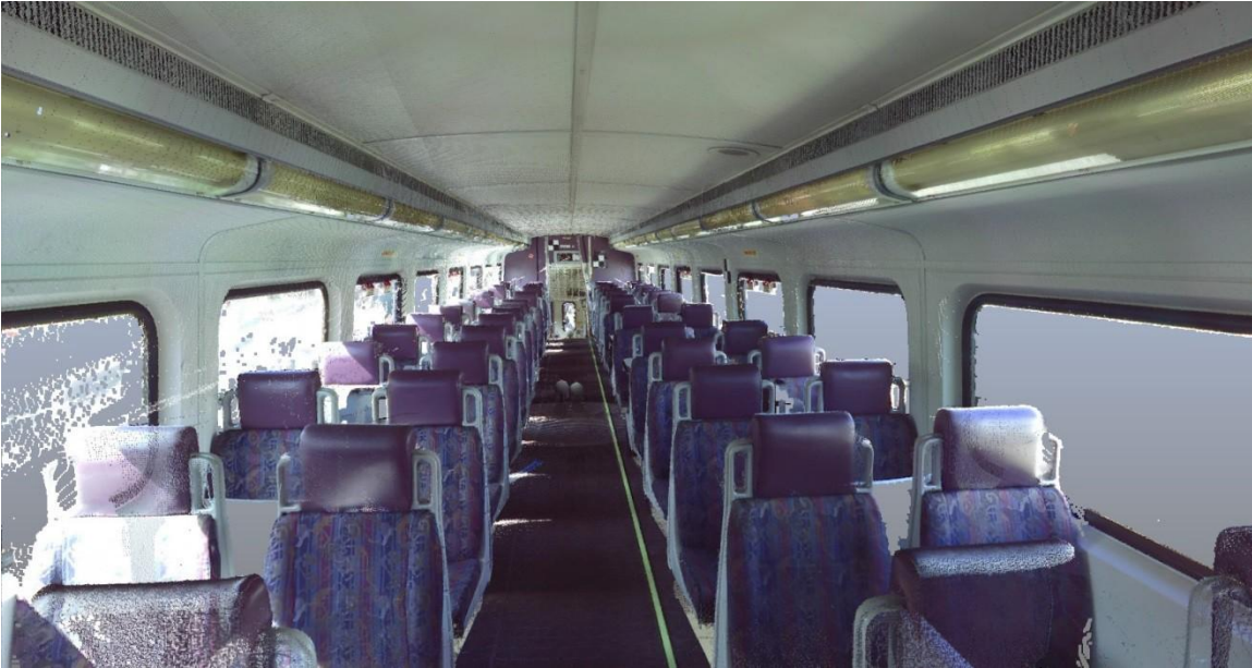
Figure 7: An image from the 3D laser scanner point cloud showing the interior of the 2 nd rail car – 206 (upper level).
