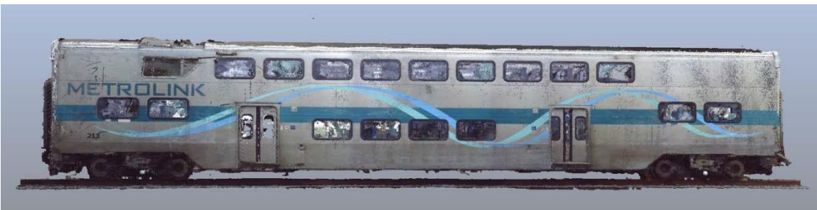
Figure 8: An image from the 3D laser scanner point cloud showing left side, with the A end on the left side of the image, of the 3 rd rail car - 211.
