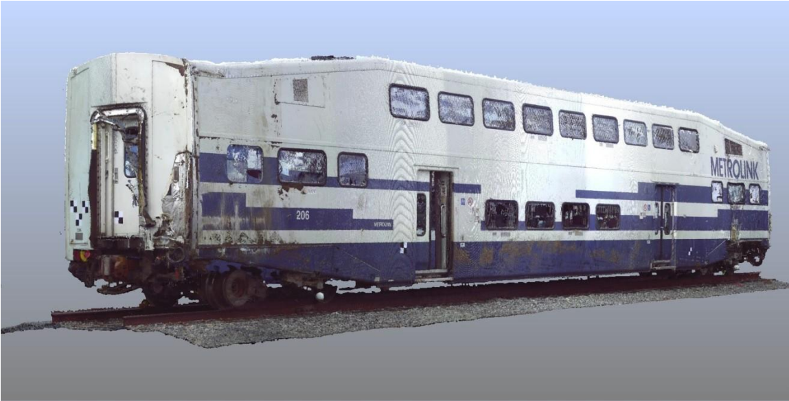
Figure 5: An image from the 3D laser scanner point cloud showing left side and the A end of the 2 nd rail car - 206.
