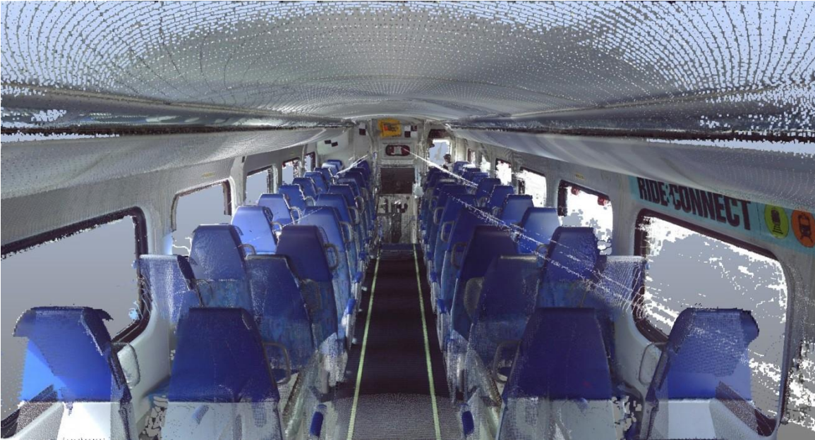
Figure 4: An image from the 3D laser scanner point cloud showing the upper level of cab car - 645.
