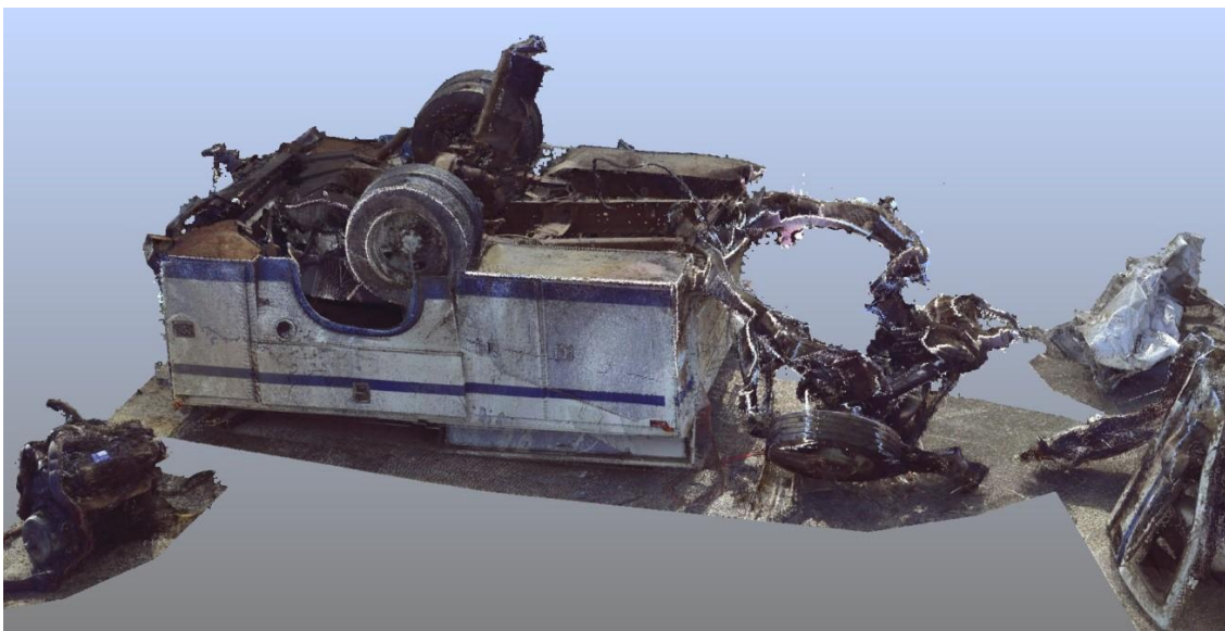
Figure 16: An image from the 3D laser scanner point cloud showing left side of the box portion of the Ford F450.
