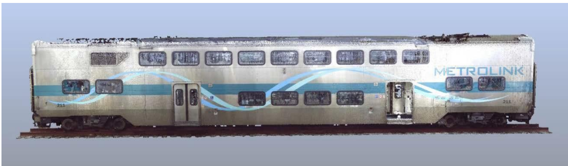
Figure 10: An image from the 3D laser scanner point cloud showing the right side, with the A end on the right side of the image, of the 3 rd rail car - 211.
