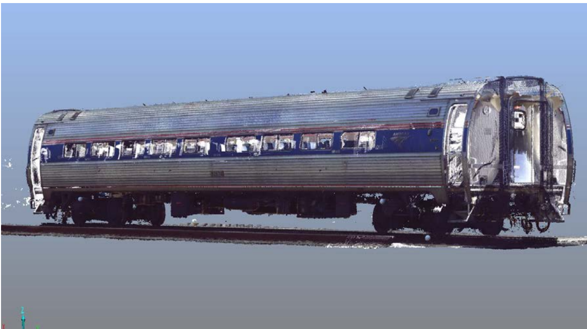
Figure 19. An image from the 3D laser scanner point cloud showing the A-end of passenger Car 82674.
