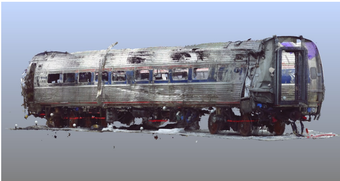
Figure 17. An image from the 3D laser scanner point cloud showing the A-end of passenger Car 3.
