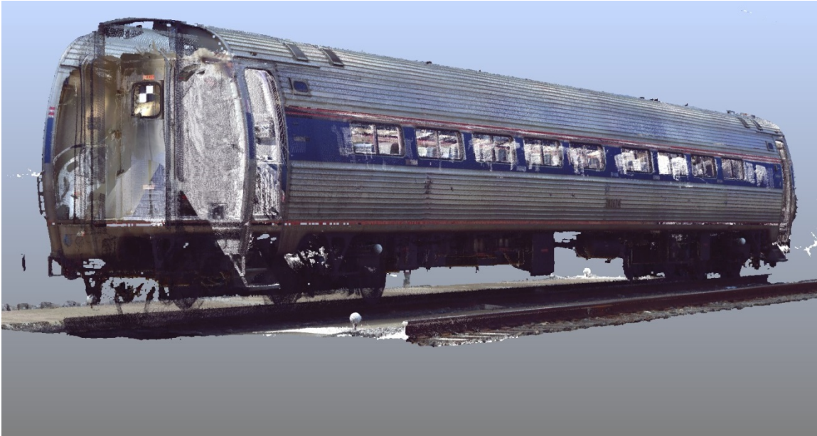
Figure 18. An image from the 3D laser scanner point cloud showing the B-end of passenger Car 82674.
