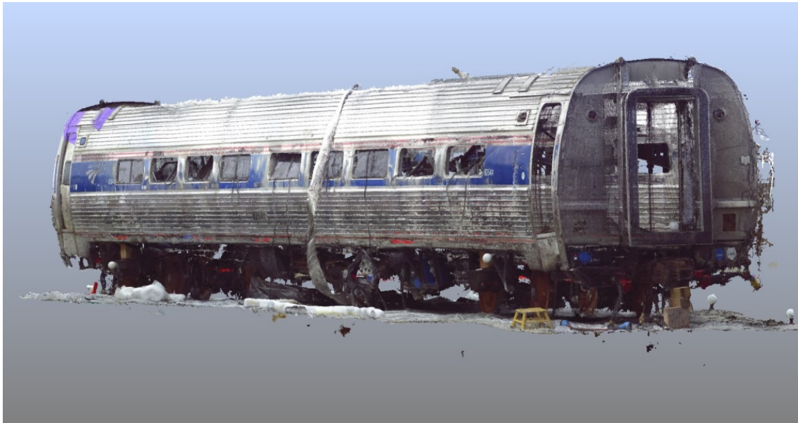
Figure 16. An image from the 3D laser scanner point cloud showing the B-end of passenger Car 3 from the other side.
