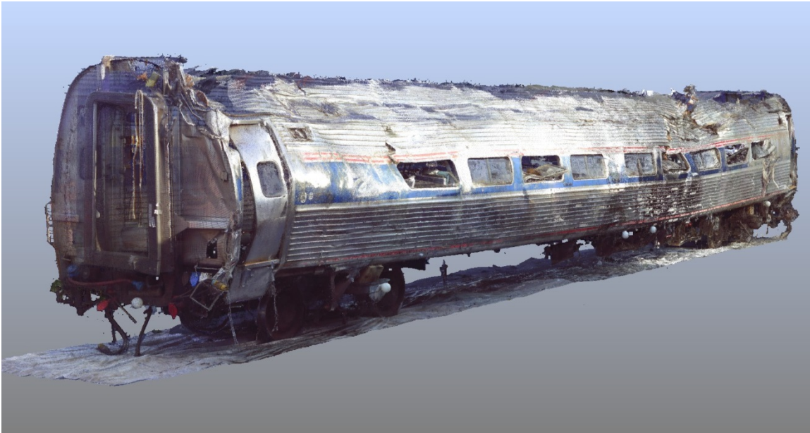
Figure 14. An image from the 3D laser scanner point cloud showing the A-end of passenger Car 2.
