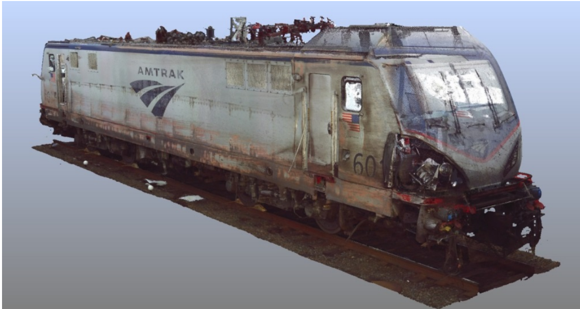
Figure 7. An image from the 3D laser scanner point cloud showing the front right of the locomotive.
