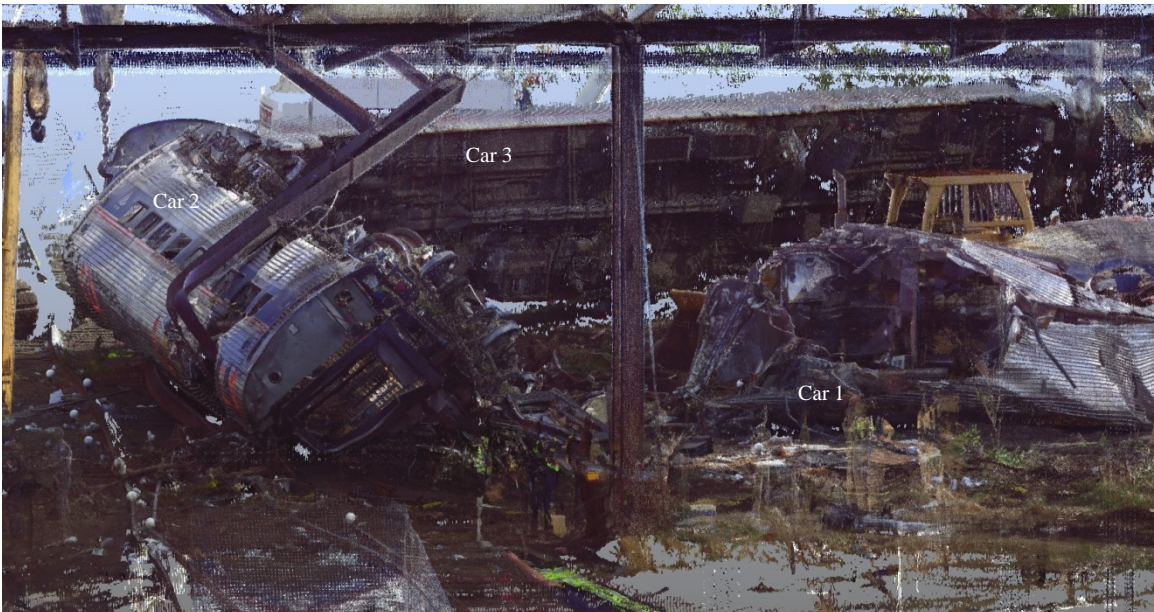
Figure 2. An image from the 3D laser scanner point cloud showing the passenger Car 2 on the left and a portion of passenger Car 1. The underside of passenger Car 3 can be seen in the background.
