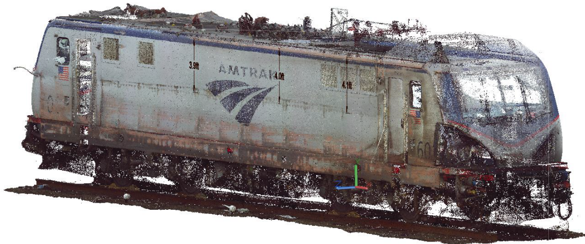
Figure 11. Measurements documenting the damage on the right side of the locomotive. The front of the locomotive is on the right side of the image. (From left to right, the dimensions are 3.9 feet, 4.0 feet, and 4.1 feet.)
