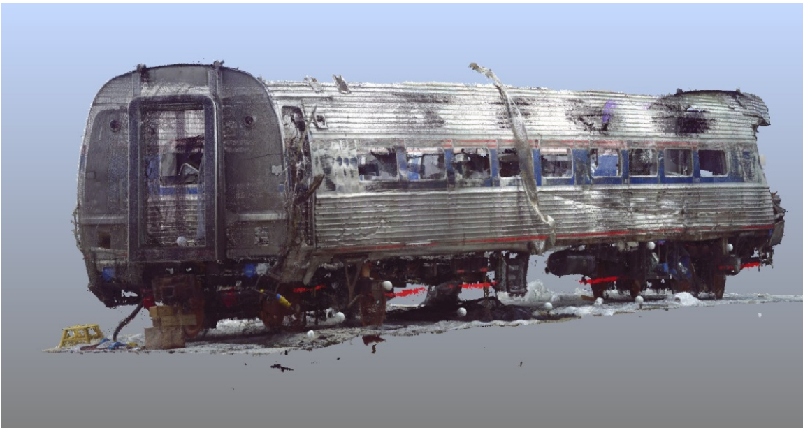
Figure 15. An image from the 3D laser scanner point cloud showing the B-end of passenger Car 3.
