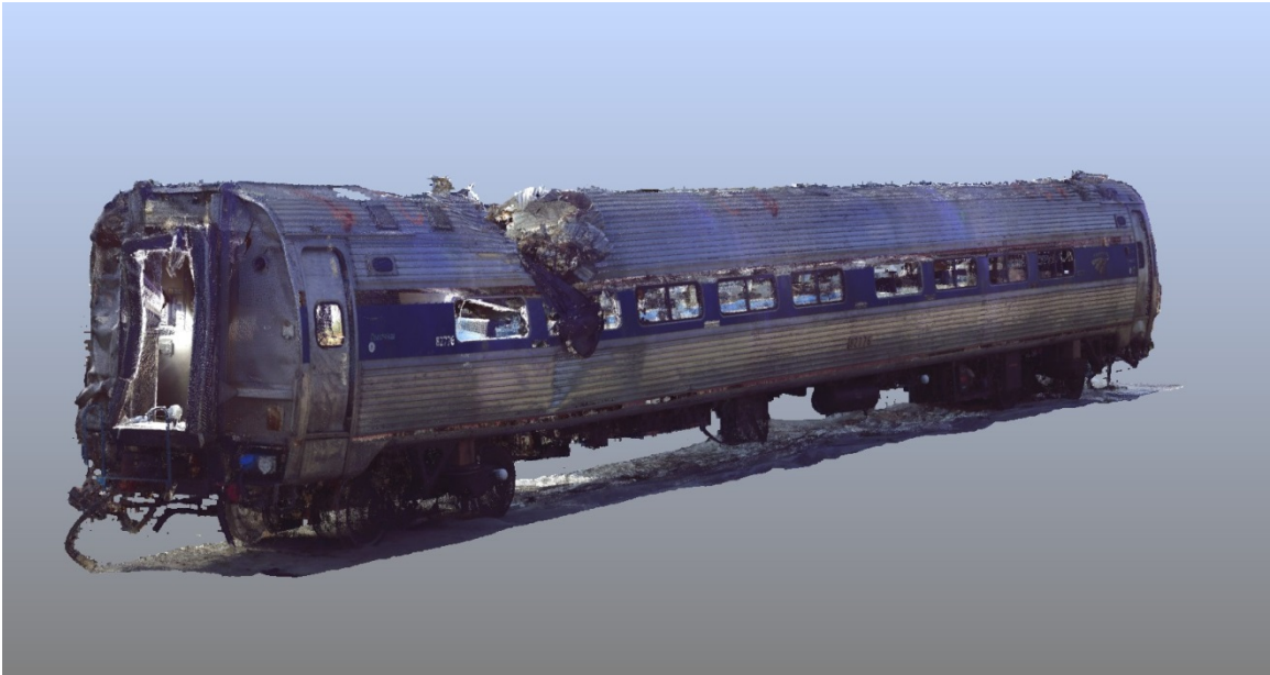
Figure 12. An image from the 3D laser scanner point cloud showing the B-end of passenger Car 2.
