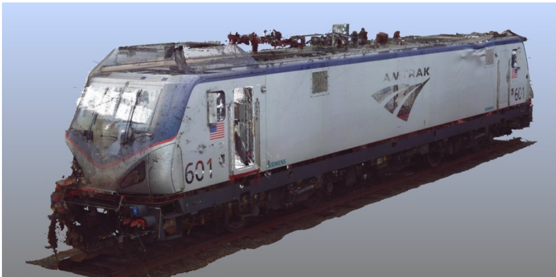
Figure 8. An image from the 3D laser scanner point cloud showing the front left of the locomotive.
