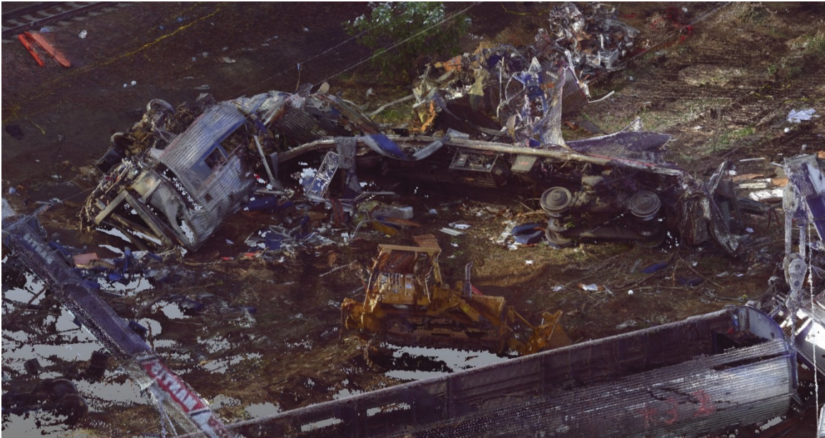
Figure 1. An image from the 3D laser scanner point cloud showing passenger Car 1 in its final rest position after vehicle extrication.
