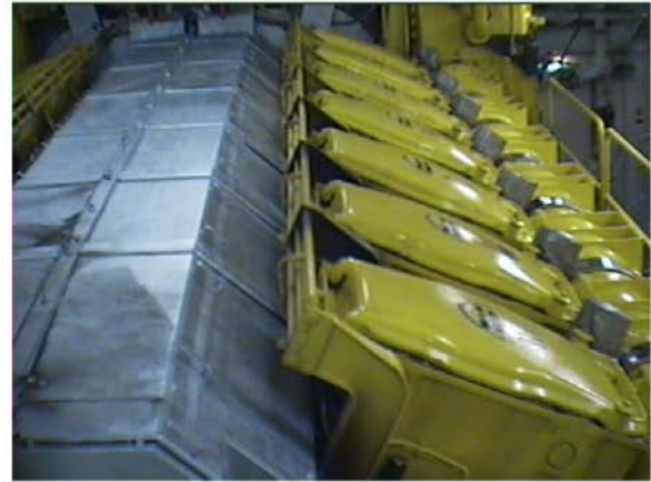
1 2 Figure 22 MAN B&W customer service bulletin thermal imagery of the first version of a V-type 48/60 3 engine. The cylinder covers and exhaust insulation is similar to the main engines on the Caribbean 4 Fantasy .
