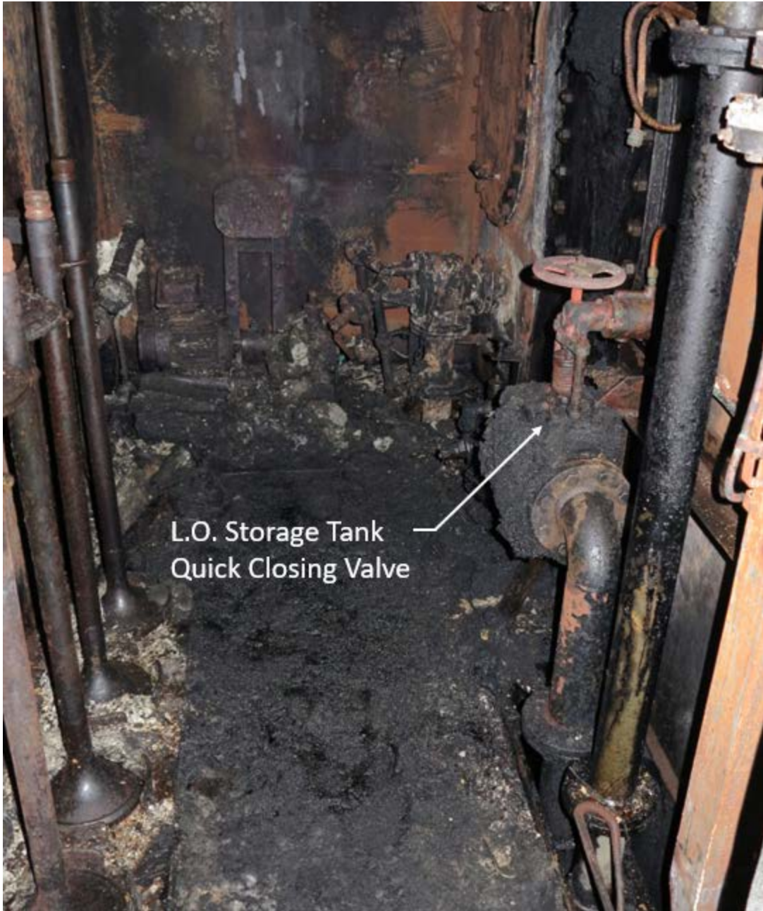
Figure 14. Port side view of the main engine room forward of engine workshop, deck 2, at frame 83. An inch and a half of lube oil is on the deck. The white arrow points to the lube oil storage tank QCV.
