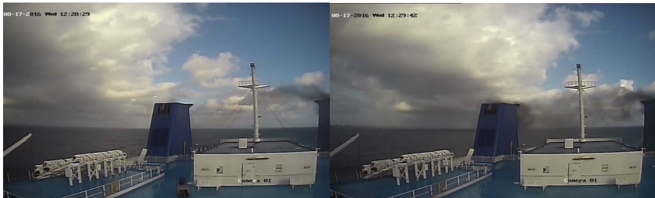
14 15 Figure 28. ECR CCTV view of the port and starboard stacks. The left frame shows the initial signs of 16 black smoke from the port funnel at 0728 local time. Note in the foreground, a crew member is in 17 process of moving one of the dogs from the kennel on this deck (deck 7) forward in preparation for 18 debarcation. On the right, about one minute later, smoke can be seen emitting from starboard stack. 19 The video at that point also showed the ship in a turn to port.
