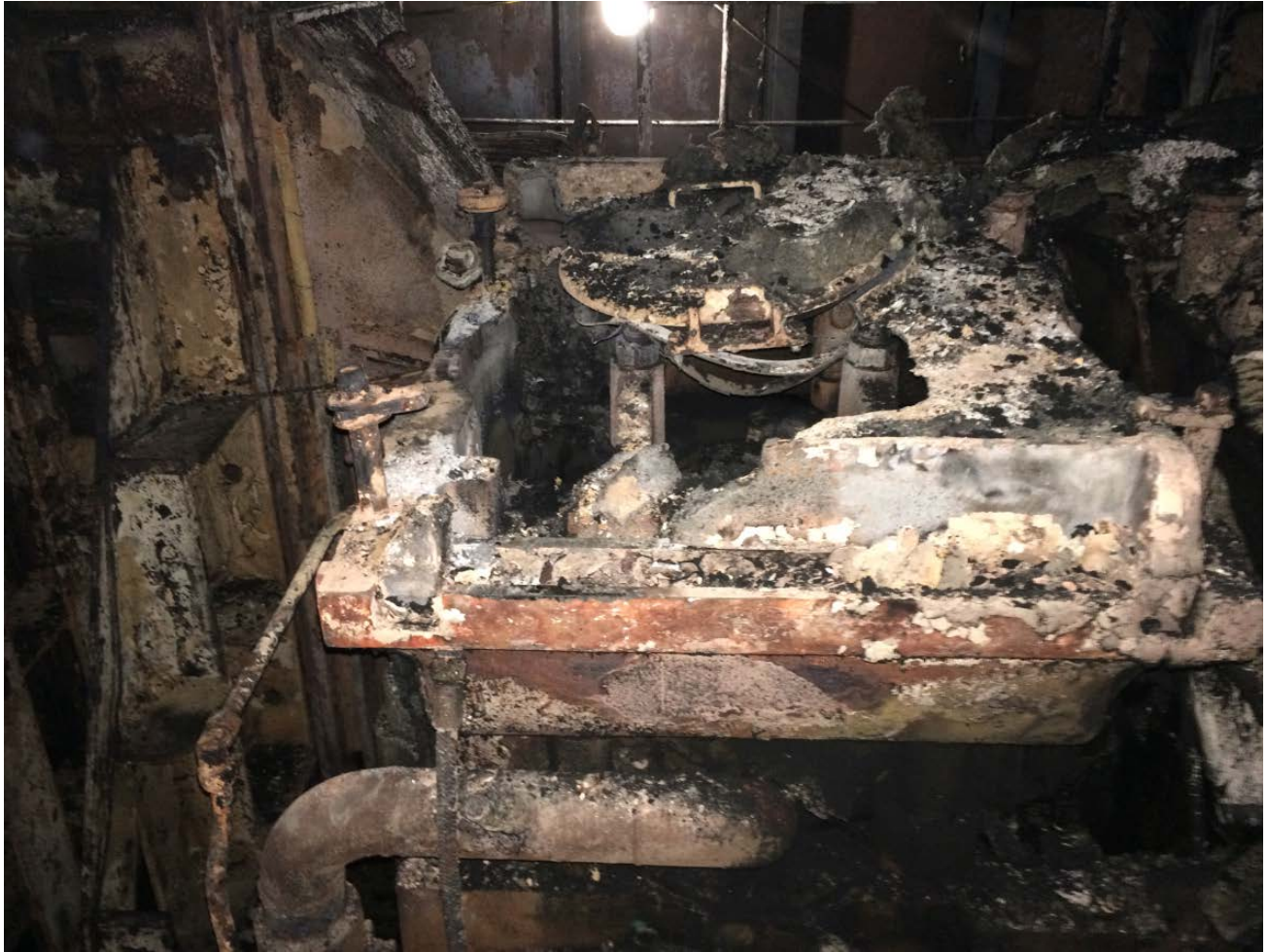
1 2 Figure 26. Caribbean Fantasy's PME cylinder no. 8. Post-accident photograph taken from the centerline 3 of the main engine room (inboard, exhaust manifold side of the PME).
