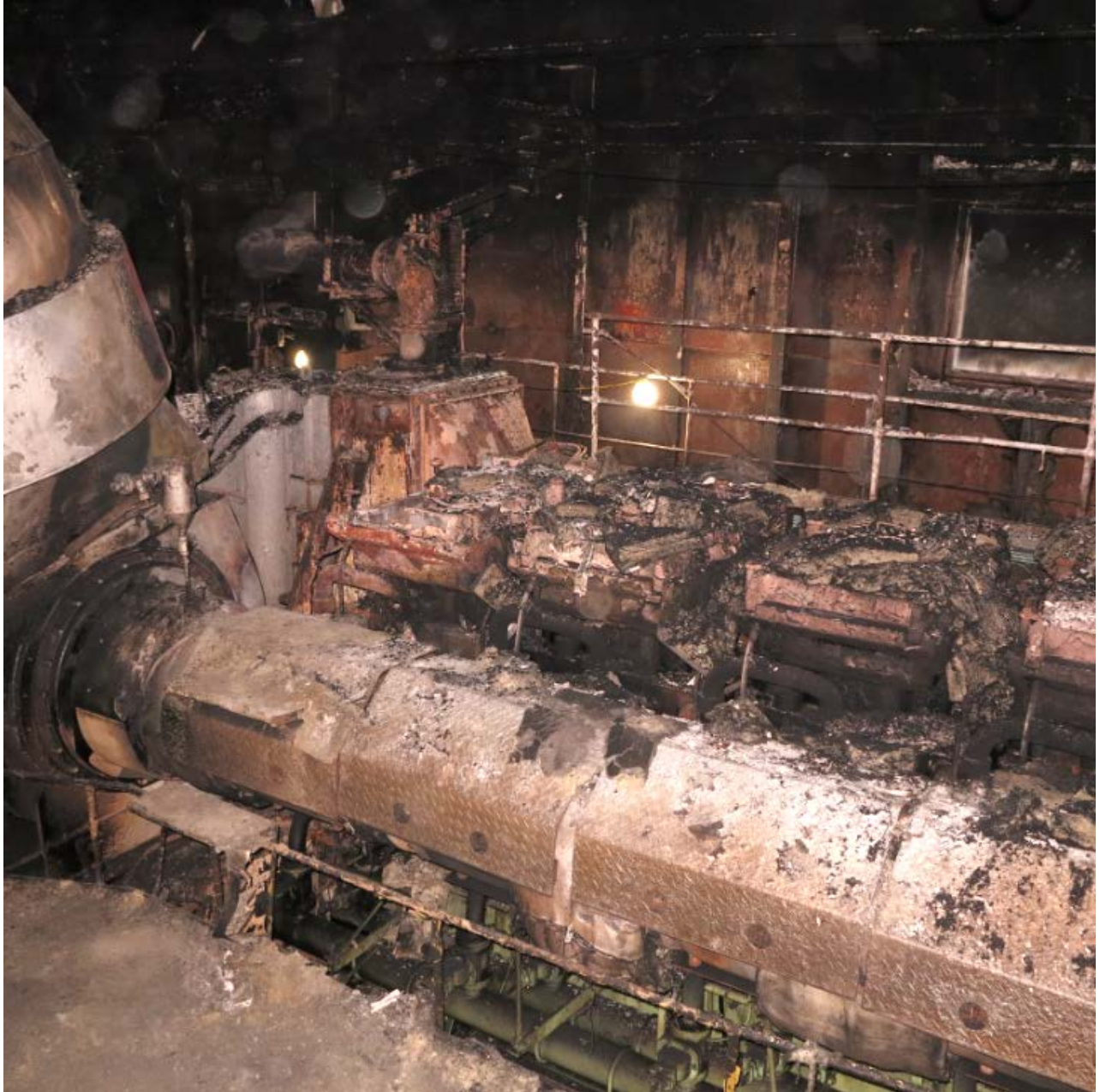
1 2 Figure 15. Caribbean Fantasy 's PME exhaust trunk manifold and turbocharger casing. Dark residual oil 3 coats the forward inboard side of the turbocharger casing and exhaust manifold lagging. Post-accident 4 photograph taken from the centerline of the main engine room (inboard side of the PME).
