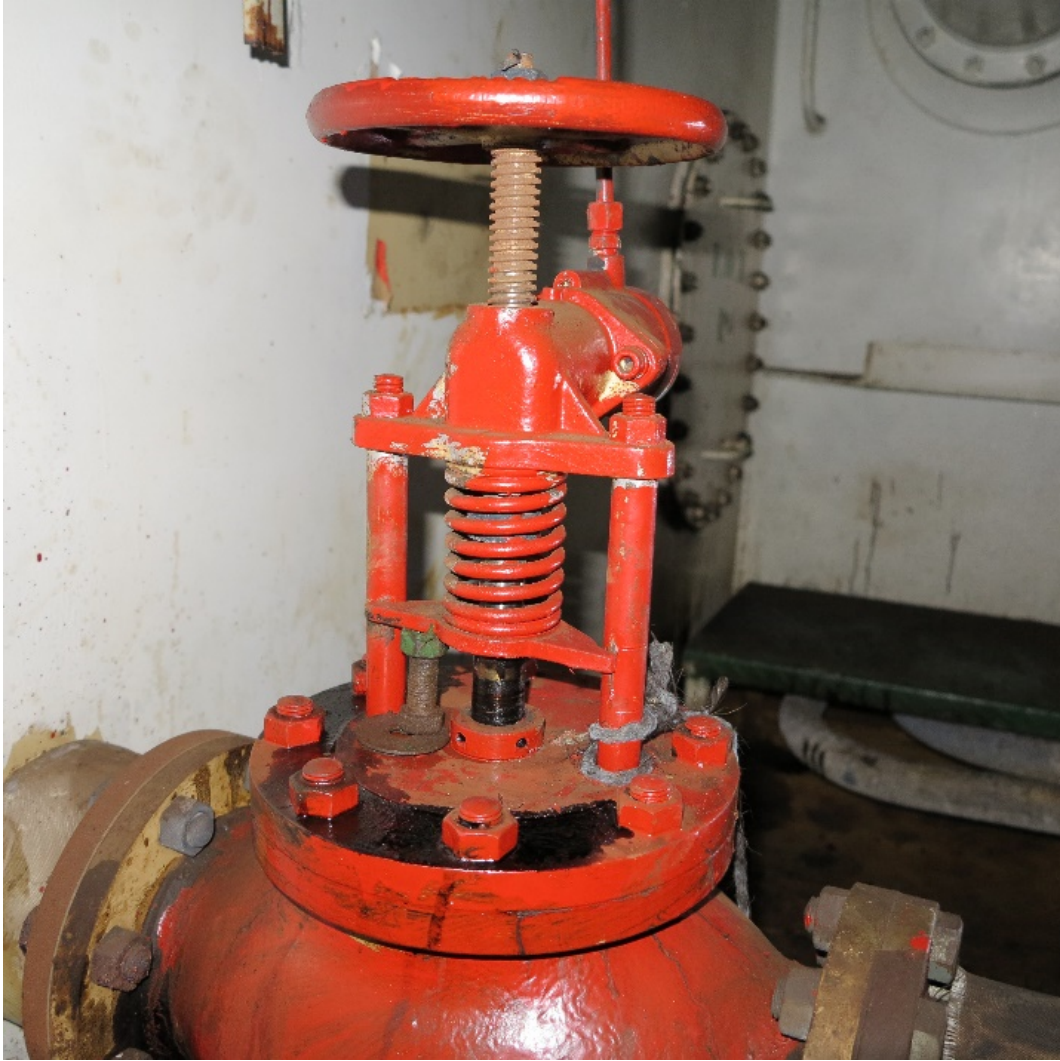
Figure 9. Caribbean Fantasy's port HFO storage tank QCV that was intentionally blocked open with a bolt, nut, and washer.
