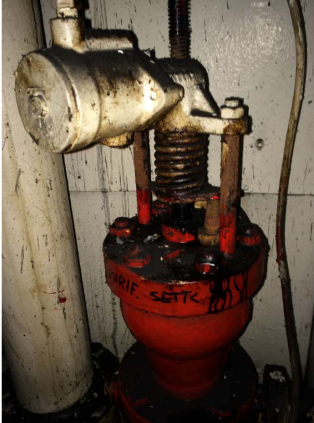
Figure 10. Caribbean Fantasy's HFO purifier settling tank starboard QCV that was intentionally blocked open with a bolt and nut.
