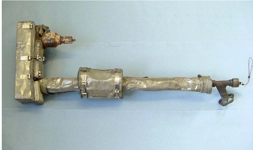
Figure 1: Indicator pipe with insulation. Satisfactory condition after 6 276 operating hours on a 14V 48/60 engine
