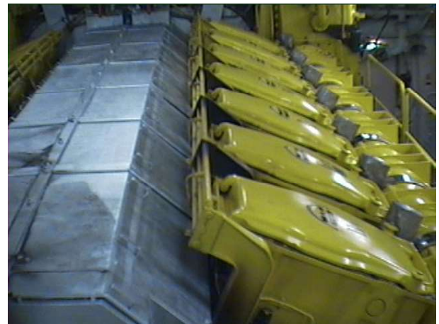
Figure. Covering of the exhaust pipe and cylinder head cover (shots taken with and without thermoscan camera)
