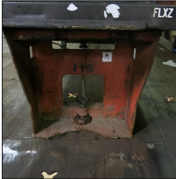
1 2 Figure 9. Front end of trailer on top of Roloc box, with Roloc fitted to button on deck (photo taken 3 on El Yunque ).
