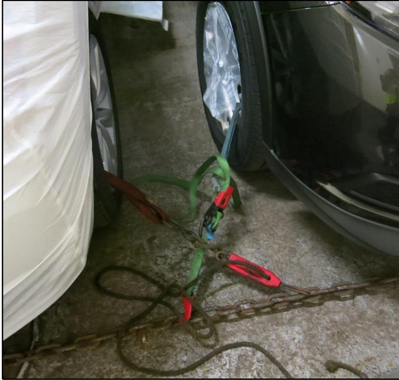
Figure 15. Lashings for two vehicles connected to one chain ( El Yunque ).
