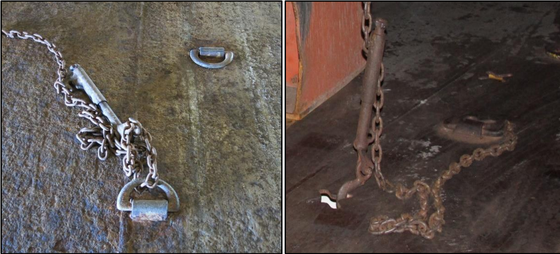
4 5 Figure 11. Left: two D-rings, one with lashing chain around it and the other with no attachments. 6 Right: hook secured to cloverleaf cutout (white area) in deck (photos taken on El Yunque ).
