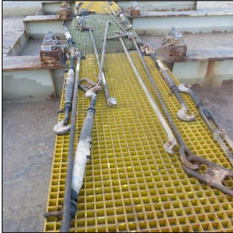
4 5 Figure 5. Foreground: lashing rods and turnbuckles for lashing containers. Background: twist 6 locks inserted into deck sockets welded to deck beams (photo taken on El Yunque ).
