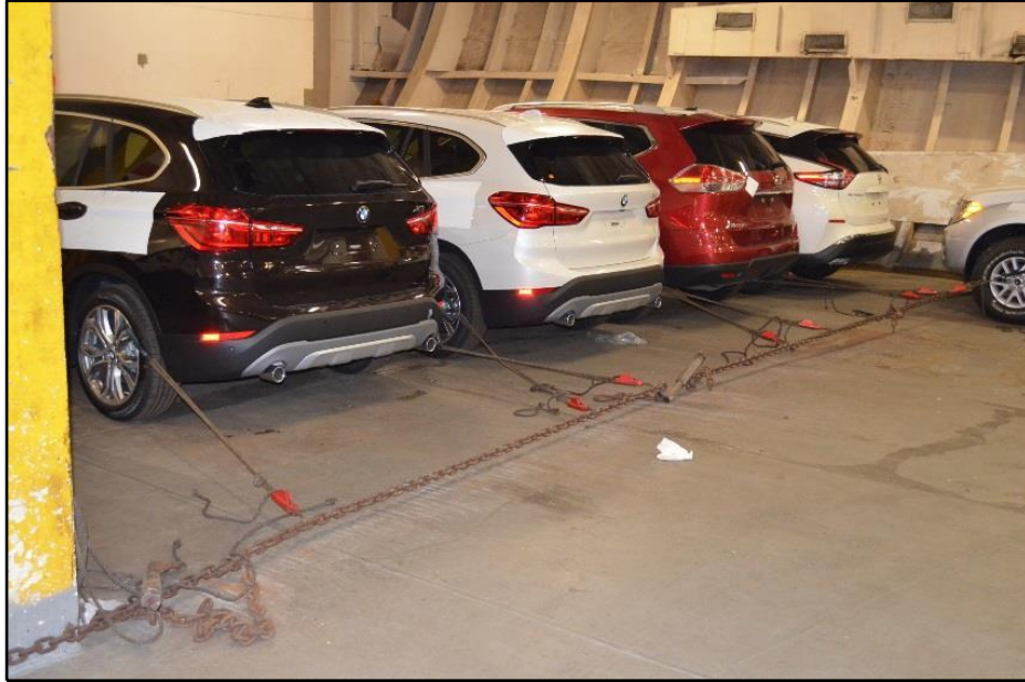
Figure 17. Two automobiles lashed to one length of chain (No. 5 hold of El Yunque ).
