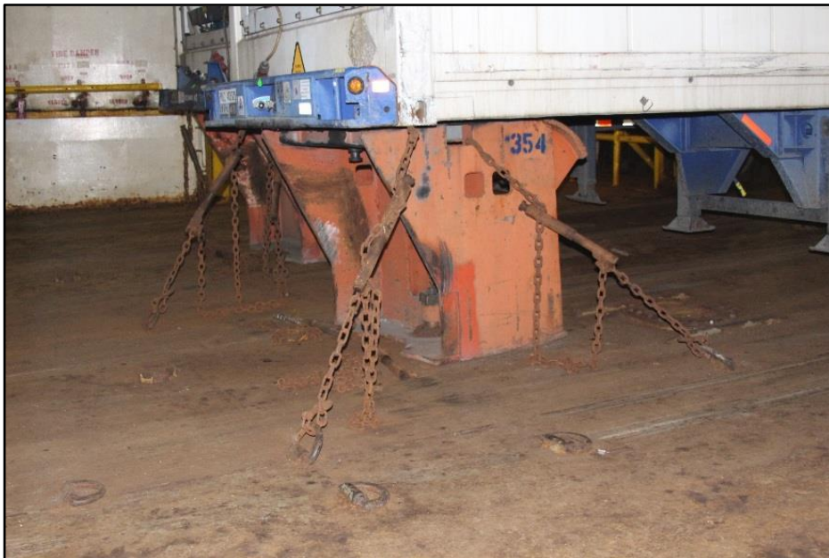
7 8 Figure 12. Chain and tensioner attached to front end of trailer and to D-rings on deck (photo taken 9 on El Yunque )
