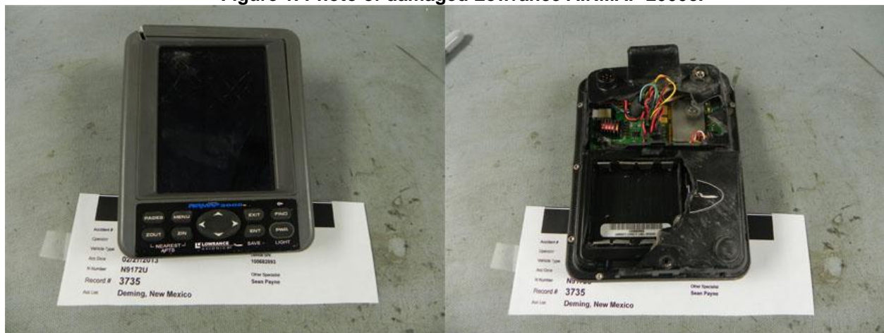
Figure 1. Photo of damaged Lowrance AIRMAP 2000c.
