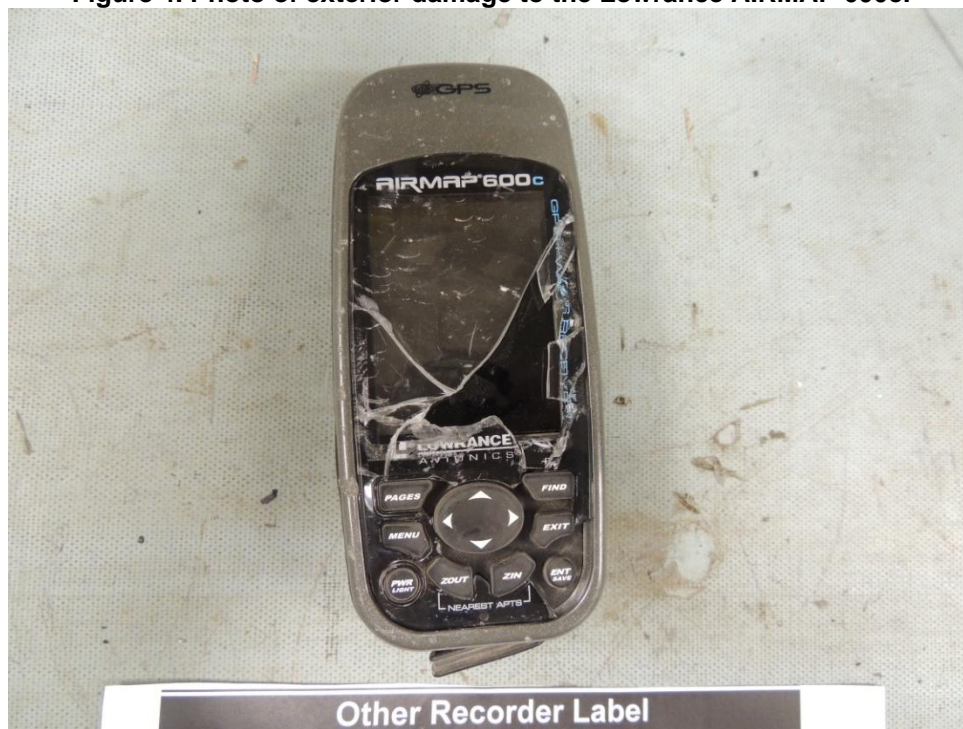
Figure 4. Photo of exterior damage to the Lowrance AIRMAP 600c.
