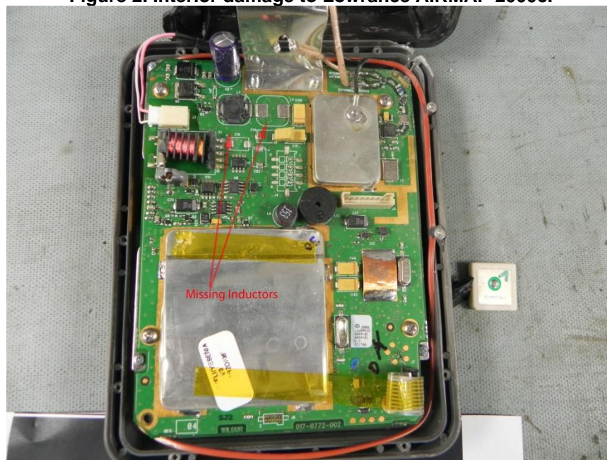
Figure 2. Interior damage to Lowrance AIRMAP 2000c.
