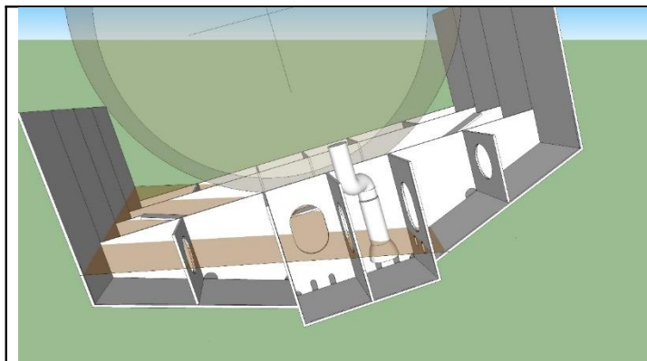
Main Sump viewed from aft with port list. Oil level at suction bell decreased relative to oil level with zero degree list.
