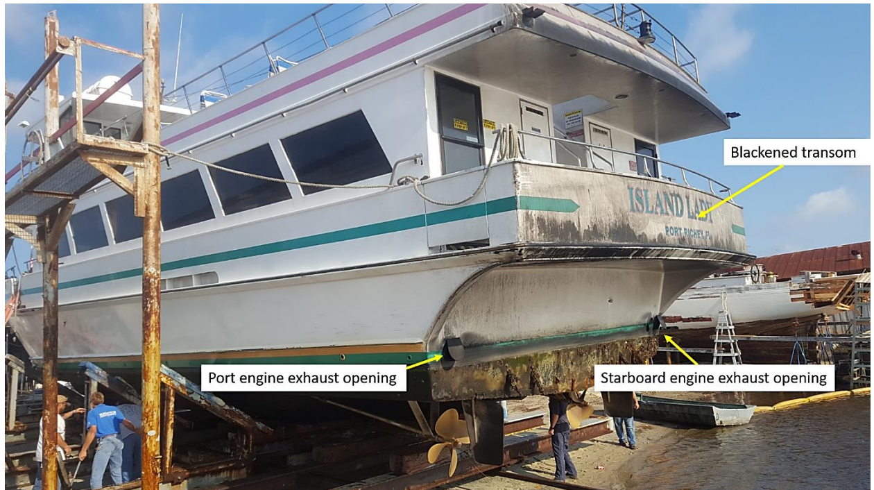
1 2 Figure 24. Stern of Island Lady while in drydock April 2017. (Photo by Coast Guard) 3
