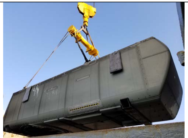
Discharging of nacelle from lower tween-deck #3 port side
