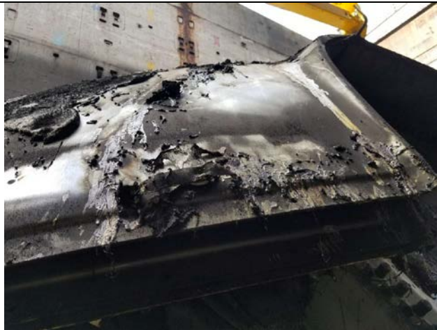
Damaged hub # 18020106 – view onto spinner shells
