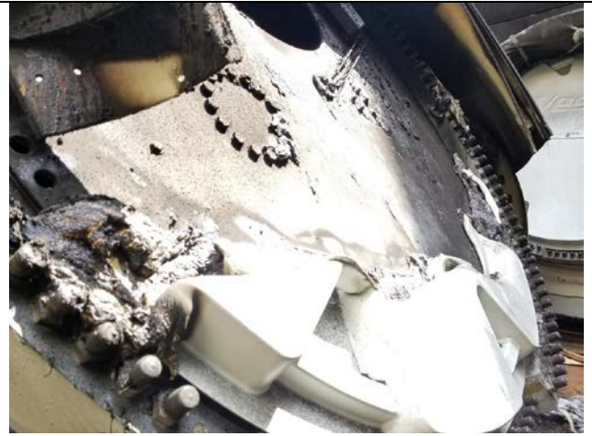
Damaged hub # 18020106 – blade flange cover molten
