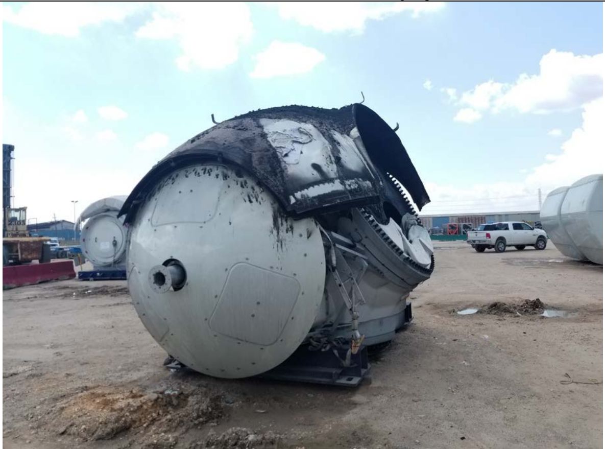
Burnt hub #18020106 at Free Trade Zone during inspection
