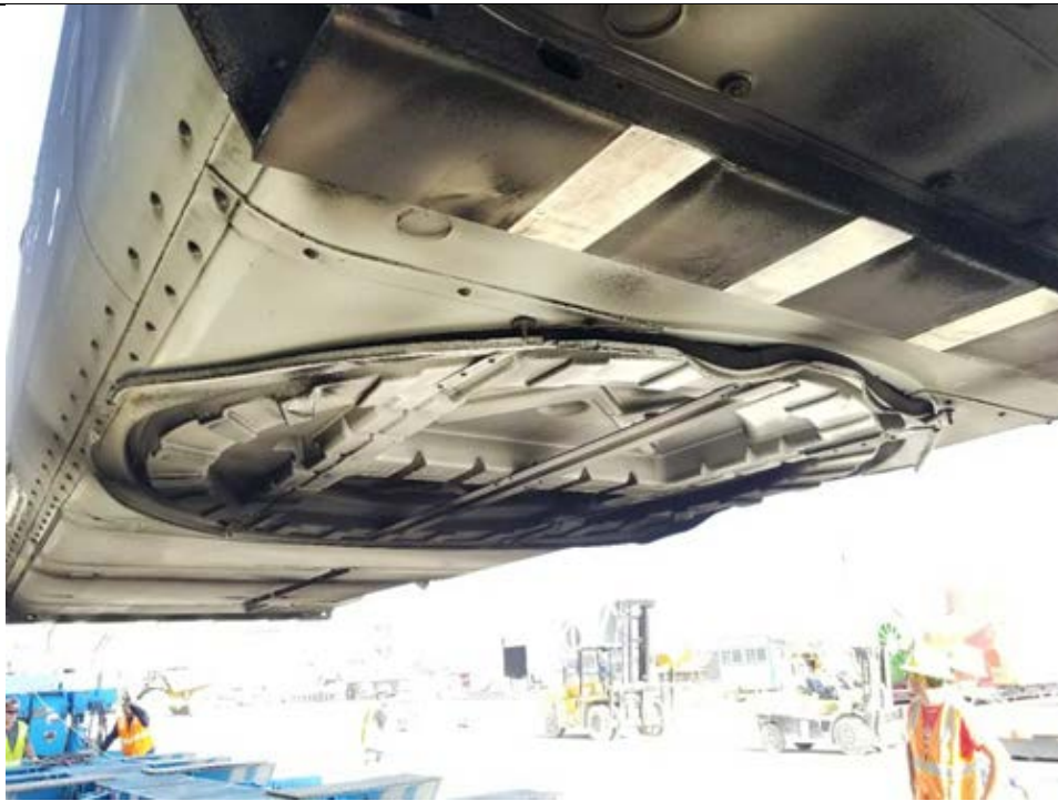
Bottom transport cover (yaw cover) of nacelle #18030052 deformed / wavy
