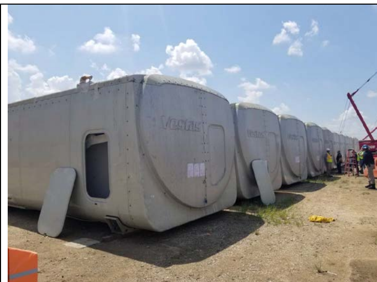
View onto lined up nacelles at the Free Trade Zone (FTZ). Eight units had been opened for a thorough interior inspection
