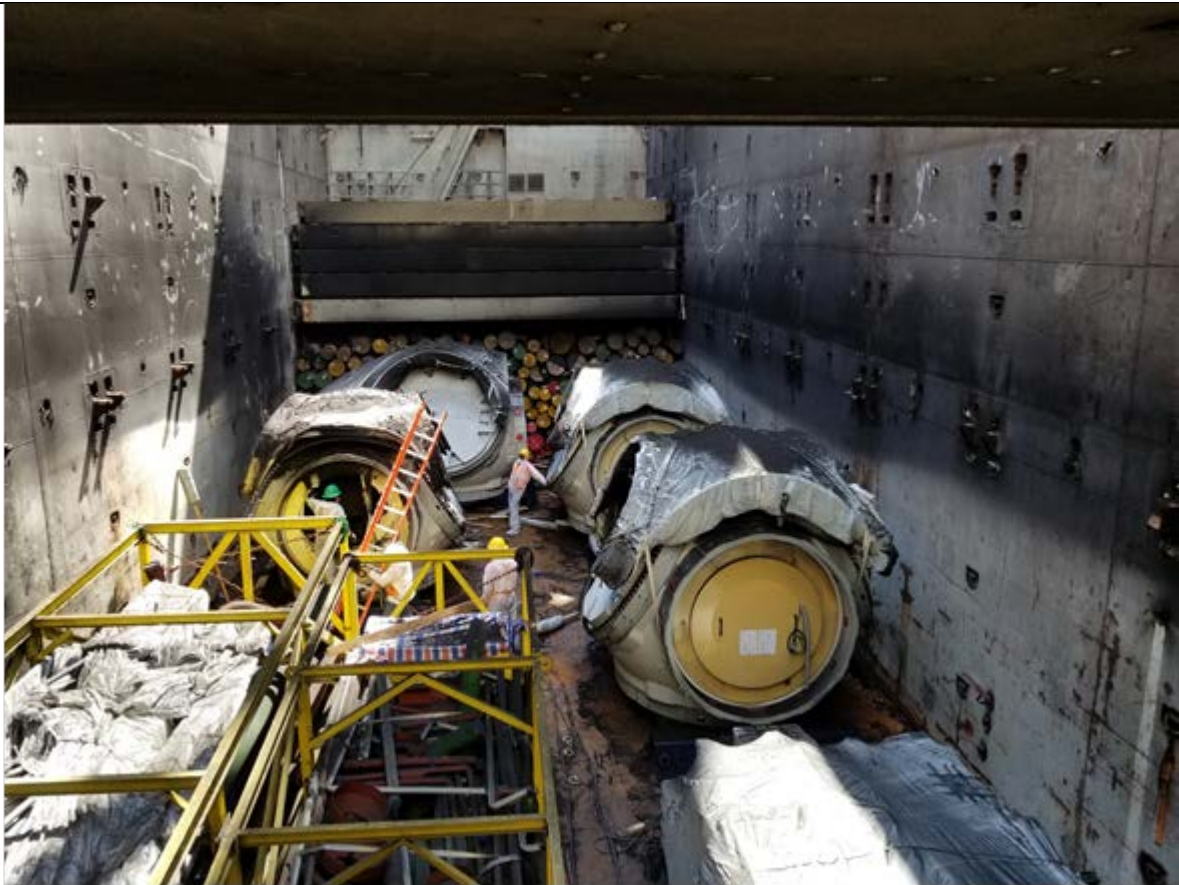
View into fire affected lower cargo hold #3 port side from forward entrance (upper tween-deck level)
