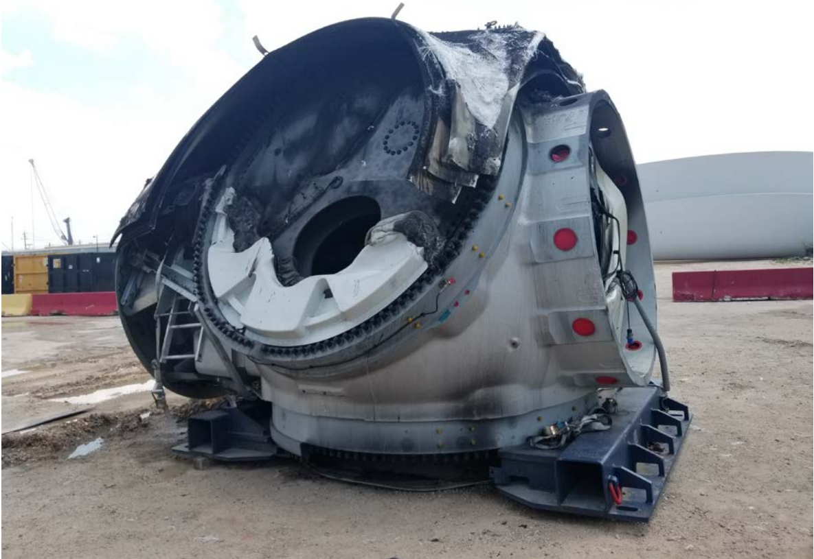
Burnt hub #18020106 at Free Trade Zone during inspection
