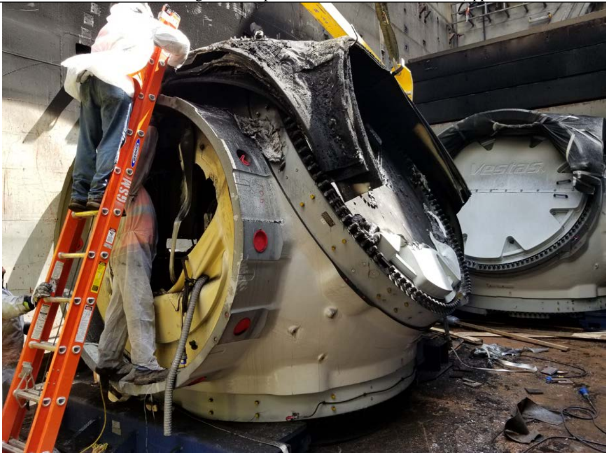
Damaged hub # 18020106 (rigging for discharge)
