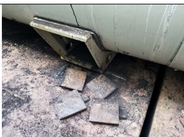
All stopper plates found cut cargo hold #3 port side
