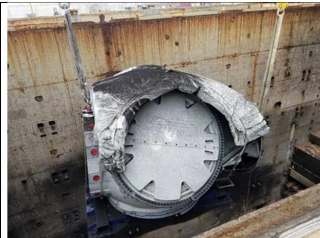
Hub #18020101 – discharged in very dirty condition
