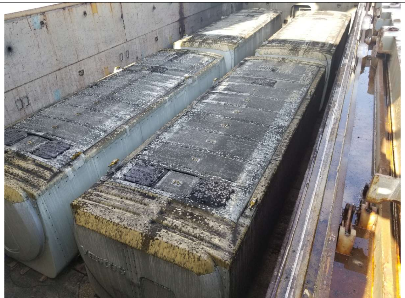
View on top of nacelles whilst stowed on the upper tween-deck of cargo hold #3 port side
