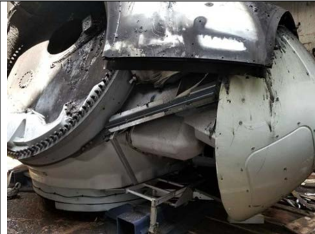
Side view onto damaged hub # 18020106
