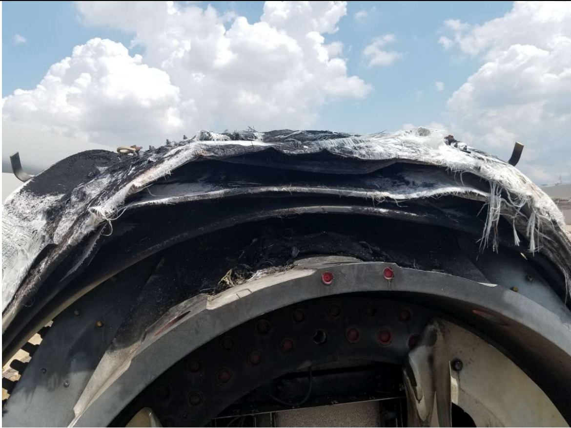
Deformed spinner shells of burnt hub #18020106
