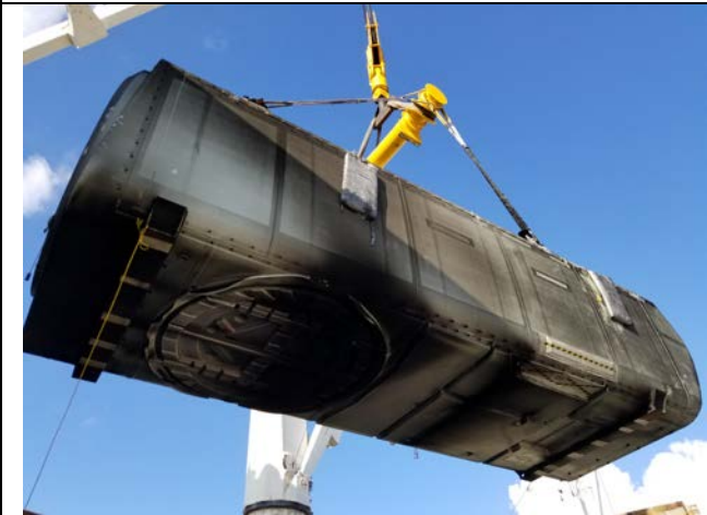
Discharging of nacelle from upper tween-deck #3 port side
