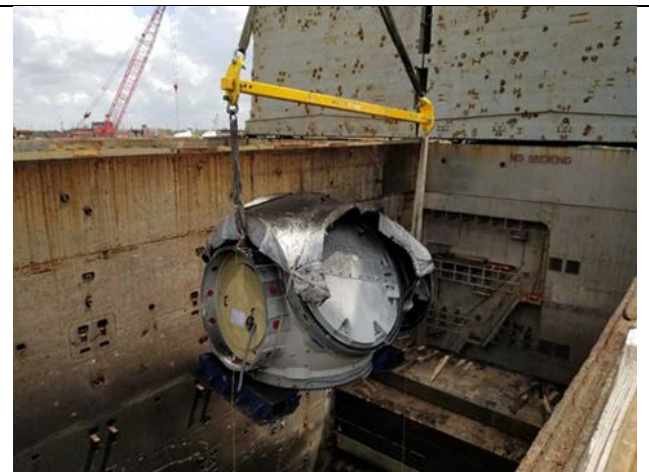
Damaged hub # 18020106 – discharged by ship's crane
