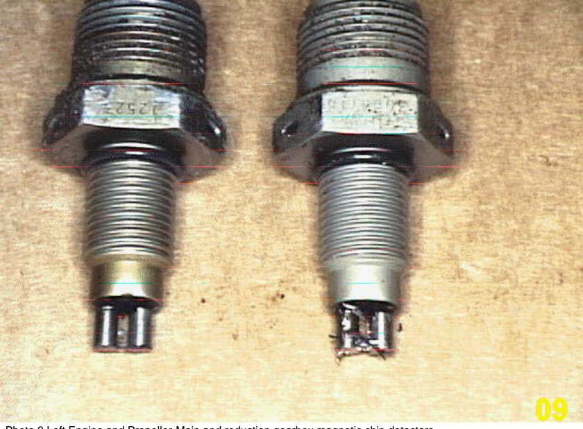
Photo 9 Left Engine and Propeller-Main and reduction gearbox magnetic chip detectors
