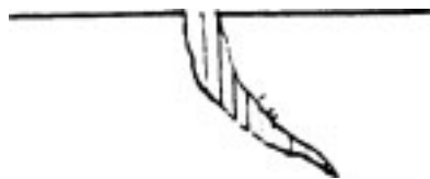
STEP 3. EXCESS PENETRANT REMOVED FROM SURFACE
