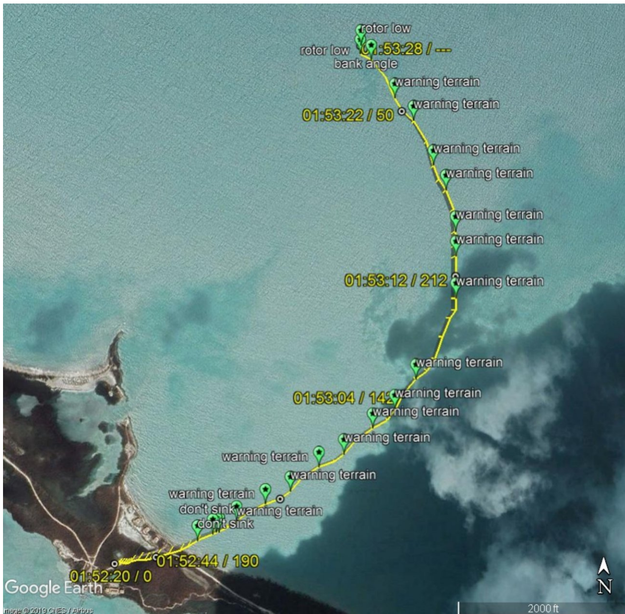
Figure 1. Cockpit announcements recorded on CVR with select times and altitudes (Figure contained in the NTSB Performance Study)
