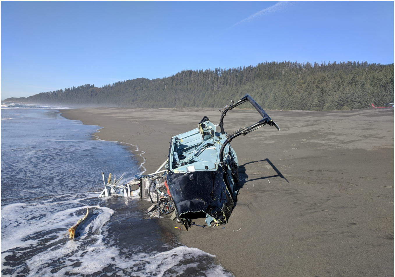
Figure 3 – Helicopter main wreckage partially embedded in the sand at low tide.
