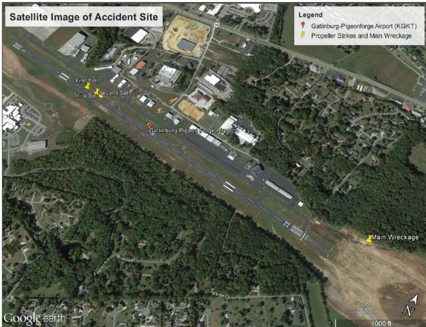
Figure 1 – Aerial image of runway 10 with the propeller strike marks and final wreckage positions annotated.
