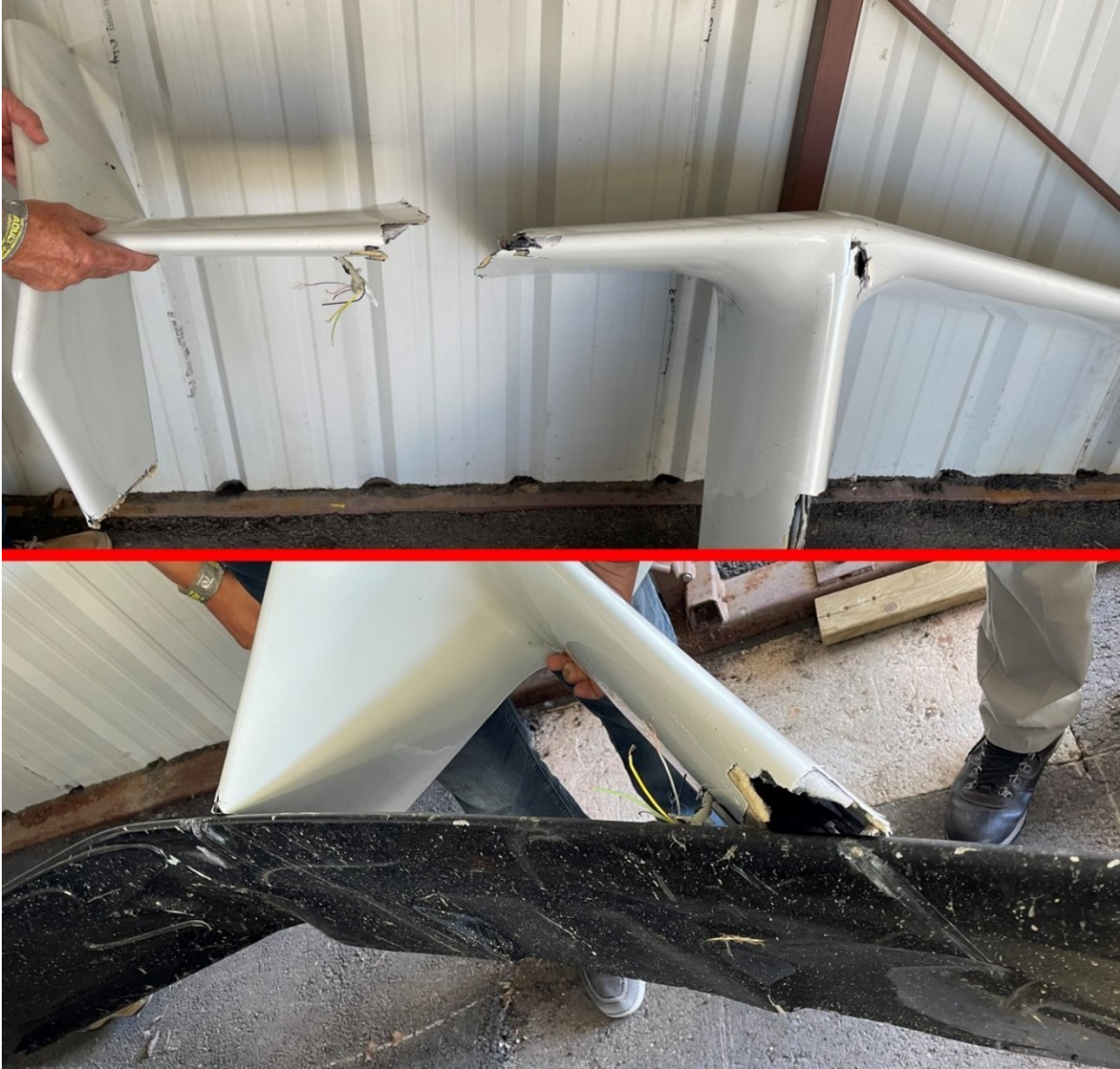
Figure 5. The upper photograph depicts the gyroplane's separated right horizontal stabilizer and lower vertical stabilizer. The lower photograph depicts the separated stabilizer section in comparison with the helicopter main rotor blade contact witness marks and white paint transfer.
