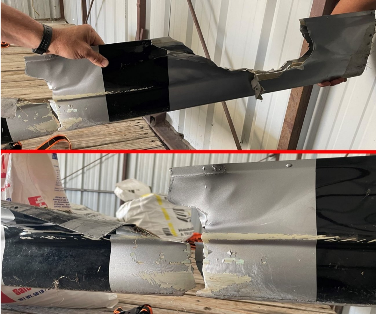
Figure 4. Separated outboard sections of the helicopter's main rotor blades.
