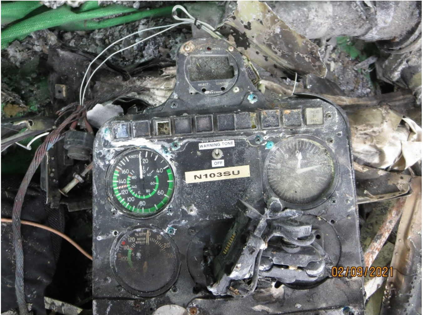
Figure 2. Instrument panel with warning tone switch (Source: MD Helicopters).
